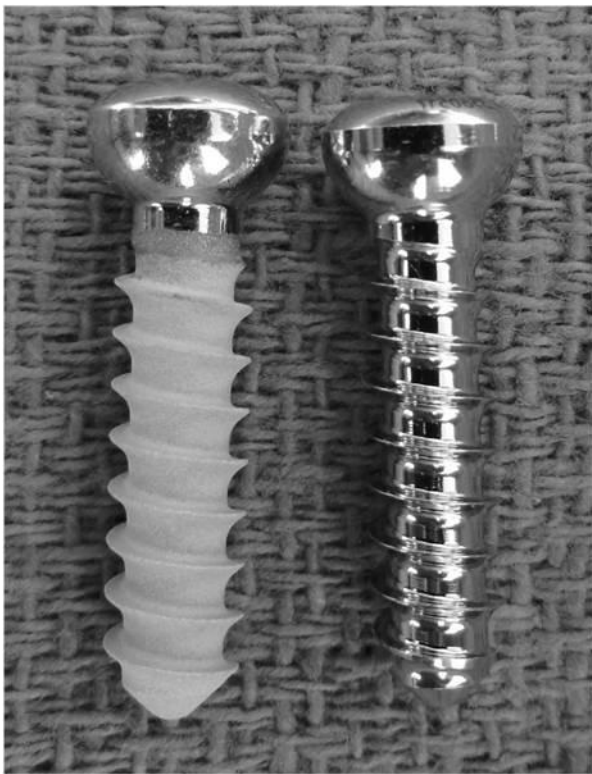
Figure 2.1. Plasma sprayed HA coated 5.5 mm AO cortical screw (left), uncoated 5.5mm AO cortical screw (right).
