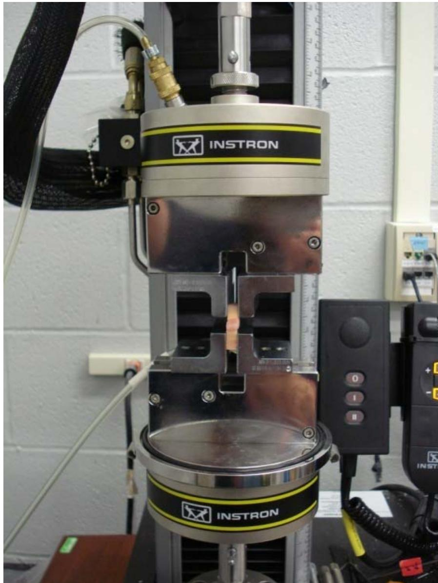
**Figure 3.2** – A laminar explant mounted in the Instron biomechanical testing device.
