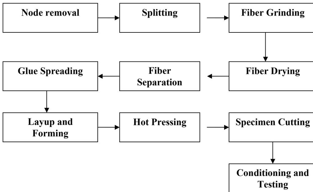
Figure 4-1. Flow chart of the fiberboard manufacturing process.
