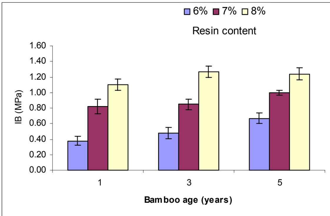
Figure 4-5. IB of fiberboards manufactured with different resin contents.
