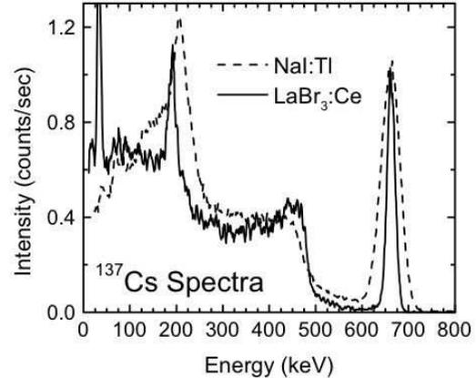
**Figure 2.** Energy spectrum of a  $^{137}\text{Cs}$  source obtained with a  $1\text{ cm}^3$   $\text{LaBr}_3$  detector. The FWHM at 662 keV is 2.6%. The comparison  $\text{NaI(Tl)}$  spectrum has an energy resolution of 6.7% (FWHM).
