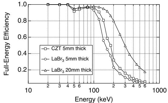
**Figure 4.** The full energy peak detection efficiency as derived from simulations of a cylindrical LaBr<sub>3</sub> scintillator of 1 cm radius and various thicknesses.
