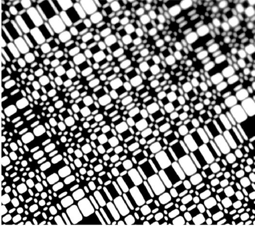
**Figure 1.** X-ray image of an etched tungsten mask obtained with a 1 mm thick CsI microfiber array and a CCD camera. The mask is a 71 x 73 URA pattern with 0.5 mm thickness and 0.5 mm minimum pixel dimensions.
