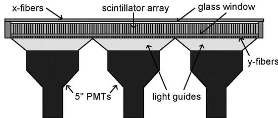
**Figure 6.** An imager design consisting of a pixellated scintillator array read out by wavelength shifting fibers. The large area PMTs are used for measuring total energy deposit. A monolithic scintillator, rather than the pixellated array, could also be used in this configuration.
