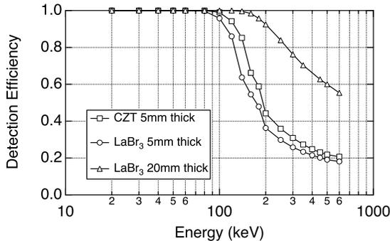
**Figure 3.** The total detection efficiency as derived from simulations of a cylindrical LaBr<sub>3</sub> scintillator of 1 cm radius and various thicknesses.
