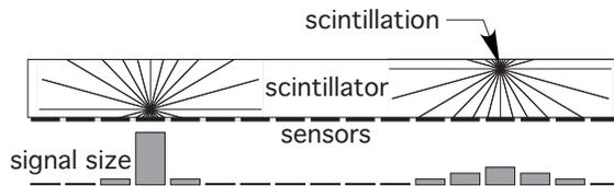
**Figure 5.** Measurement of the photon interaction depth.
