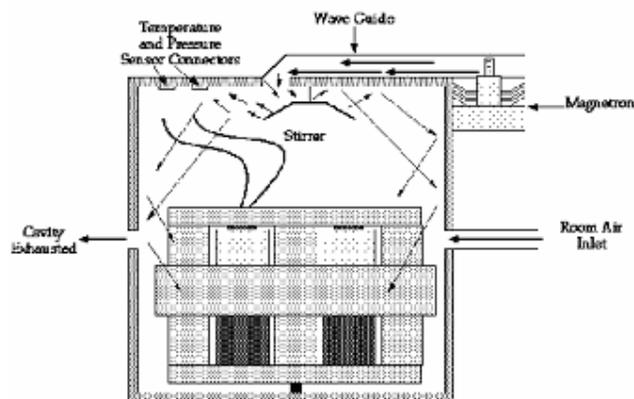
**Figure 4: Microwave-assisted Extraction Process**
