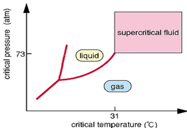
**Figure 6: Phase Diagram of Supercritical  $\text{CO}_2$**
