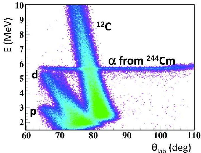
FIG. 3. (Color online) Energy versus angle measurements for protons, deuterons and  $^{12}\text{C}$  atoms scattered out of the deuterated polyethylene target, measured in a single  $\Delta E$  detector. The horizontal line corresponds to the  $\alpha$  decay of  $^{244}\text{Cm}$  present in the target chamber.
