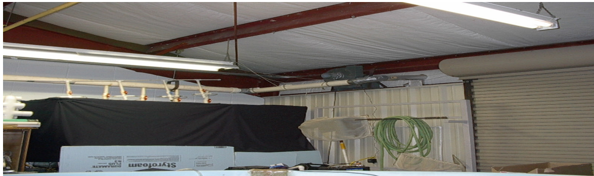
Figure 3.2 PVC pipes constructed with black cloth and hooked with fan to avoid odors of the chemicals in the laboratory.
