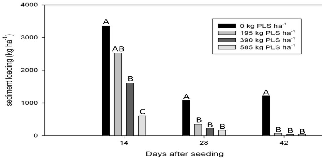
**Figure 7.** Sediment losses from swards of perennial ryegrass seeded at 0, 195, 390, or 585  $\text{kg ha}^{-1}$  and subjected to rainfall simulations 14, 28, and 42 days after seeding. Sediment loading means are separated by rainfall simulation date using Fisher Protected LSD ( $\alpha=0.05$ ).
