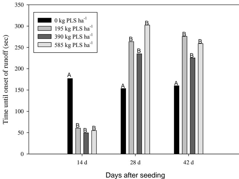
**Figure 3.** Perennial ryegrass seeding rates (0, 195, 390, and 585 kg ha<sup>-1</sup>) delay the onset of surface runoff during rainfall simulations performed at 14, 28, and 42 days after seeding. Time duration means are separated by rainfall simulation date using Fisher Protected LSD ( $\alpha=0.05$ )
