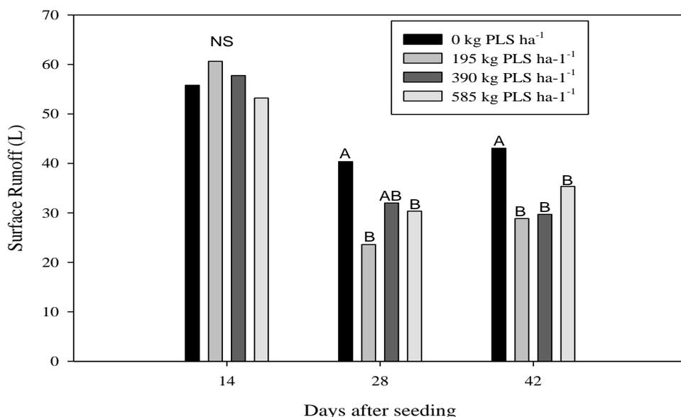
**Figure 5.** Perennial ryegrass seeding rate (0, 195, 390, and 585 kg ha<sup>-1</sup>) effects on runoff volume losses from rainfall simulations performed at 14, 28, and 42 DAS. Time duration means are separated by rainfall simulation date using Fisher Protected LSD ( $\alpha=0.05$ ).
