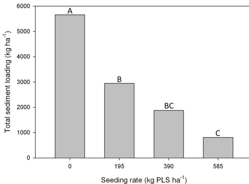
**Figure 9.** Total sediment loading from three rainfall simulations conducted 14, 28, and 42 days after seeding on perennial ryegrass swards seeded at 0, 195, 390, or 585 kg ha<sup>-1</sup>. Sediment loading means are separated by rainfall simulation date using Fisher Protected LSD ( $\alpha=0.05$ ).
