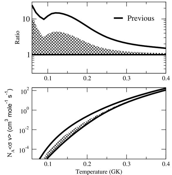
**Fig. 4.** The top panel shows the ratio of the  $^{18}\text{F}(p, \alpha)^{15}\text{O}$  rate to the previously-calculated minimum rate [19] while the bottom panel shows the individual rates directly. The previous uncertainty band is outlined with solid lines, and the reduced uncertainty band from the current work is shown in white. The previous upper limit agrees with the current result, but the lower limit has been increased by a factor of 1.5–4.
