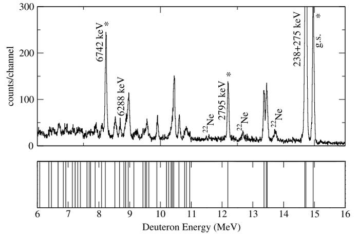
**Fig. 1.** The top panel shows the observed deuteron energy spectrum at  $29^\circ$  while the bottom panel shows the expected energies for the population of known levels in the  $^{20}\text{Ne}(p, d)^{19}\text{Ne}$  reaction at the same angle and a bombarding energy of 30 MeV. Peaks labeled with stars were used for energy calibration.
