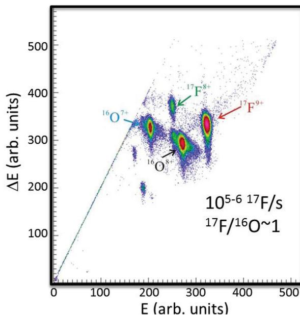
Figure 2: (color online) A particle identification spectrum taken to assay the secondary beam. Multiple charge states with the same magnetic rigidity and transported by *TwinSol* to the secondary target. A small amount of N and C was also observed.
