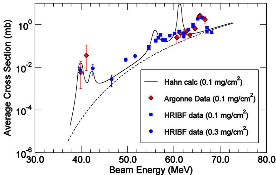
Figure 1: (color online) Previous  $^{17}\text{F}(\text{p},\alpha)^{14}\text{O}$  measurements. The HRIBF data are from Blackmon et al. 2001, and the Argonne data are from Harss et al. 1999. The target thickness is indicated in the legend. The solid curve is a prediction based upon resonance parameters from Hahn et al. 1996 averaged over the energy loss in the target.
