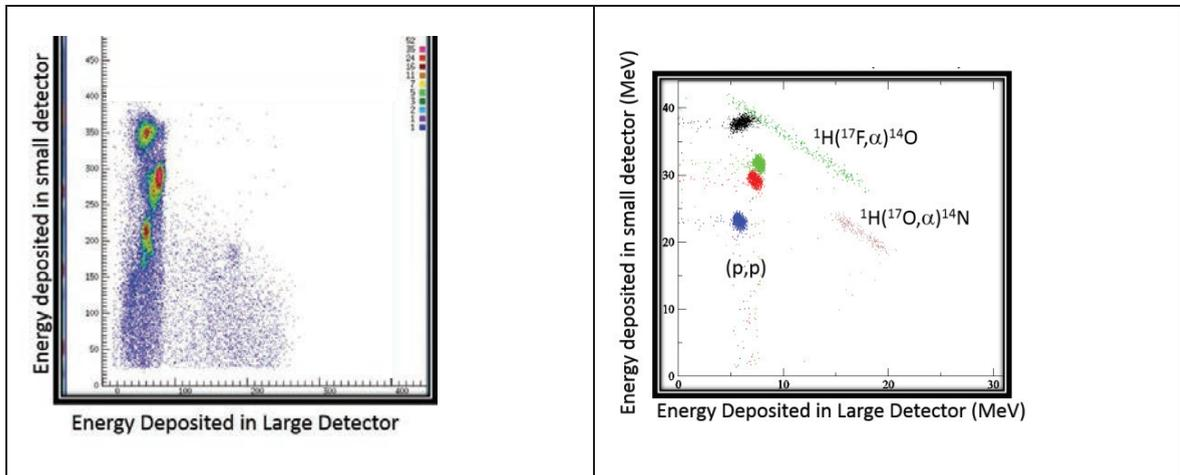
Figure 4: (color online) Left: Data similar to Fig. 3 taken with the secondary  $^{17}\text{F}$  beam on a  $\text{CH}_2$  target. Right: A simulation of the expected energies of groups produced by various reactions.
