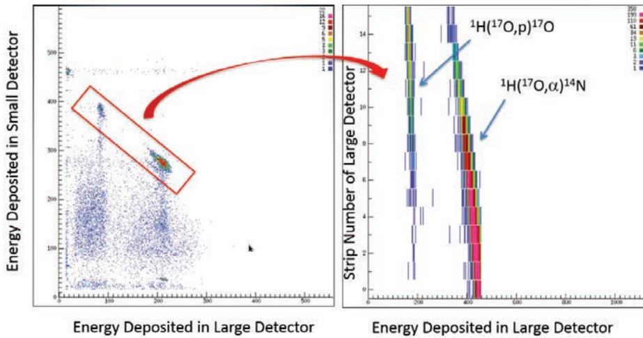
Figure 3: (color online) Data taken with an  $^{17}\text{O}$  beam on a  $\text{CH}_2$  target. Events from the  $^1\text{H}(^{17}\text{O},\text{p})^{17}\text{O}$  and  $^1\text{H}(^{17}\text{O},\alpha)^{14}\text{N}$  reactions are cleanly identified.
