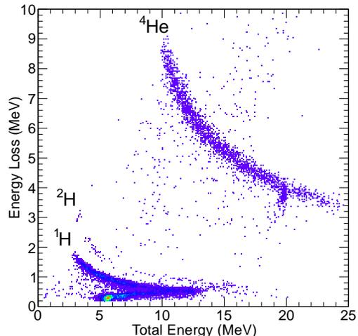
FIG. 6. Light charged particles identified in the  $\Delta E-E$  silicon detectors according to their characteristic energy-losses and selected by gating on incident  $^{17}\text{F}$  beam particles, identified through the time-of-flight analysis displayed in Fig.5
