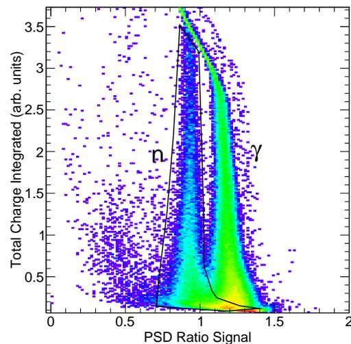
FIG. 3. Neutron pulse-shape discrimination spectrum for a single RESONEUT detector, representing  $\gamma$ - and neutrons emitted from a  $^{252}\text{Cf}$  source. Also drawn is a gate used to select neutron-based events in the analysis.
