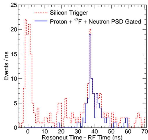
FIG. 10. Time-of-flight (tof) signals of neutron-detection analyzed relative to the accelerator RF reference for  $^{17}\text{F}$ -based events triggered by a silicon-detector. Shown is the raw distribution, including the  $\gamma$ -based events at 0.6 ns tof, and the events detected in coincidence with an identified proton, heavy ion and applied  $\gamma$ -discrimination through the pulse-shape analysis.
