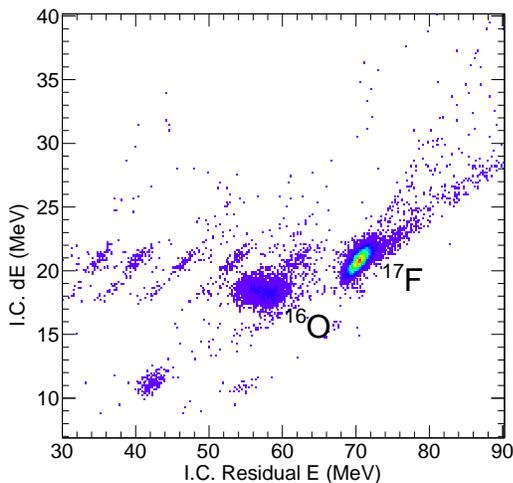
FIG. 4. Sample beam composition observed in the gas ionization chamber, characterized according to the partial energy loss (dE) and residual energy  $E$  detected in the active sectors of the chamber, but excluding the position-resolving sections. This spectrum represents data taken without the  $\text{CD}_2$  target. During the experiment the beam composition was continuously sampled at a 1/1000 downscaled trigger rate.
