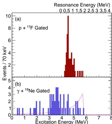
FIG. 12. The excitation energies of the states populated by the  $(d, n)$  reaction reconstructed using the neutron time-of-flight measurement (see text). Panel (a) Events detected in coincidence with a proton and a  $^{17}\text{F}$  reaction residue. Panel (b) Events detected in coincidence with a  $\gamma$ -ray and a  $^{18}\text{Ne}$  reaction residue. The dashed line displayed in Panel (b) represents an upper limit estimate for events from uncorrelated background in the time spectra.
