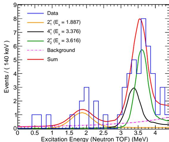
FIG. 13. The observed spectrum compared with three peaks at the locations of the  $^{18}\text{Ne}$  bound states  $2_1^+$ ,  $4_1^+$  and  $2_2^+$ . The peak areas are consistent with expectations from the simulation based on the spectroscopic factors from the mirror reaction [17].
