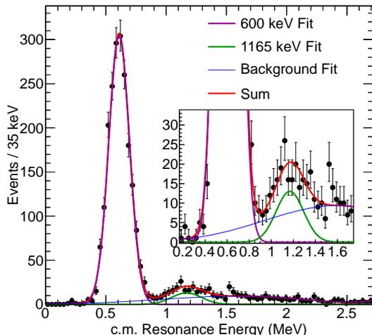
FIG. 8. Center-of-mass resonance-energy spectrum reconstructed from the invariant-mass analysis of the detected coincident proton+ $^{17}\text{F}$  events. The spectrum is dominated by a peak at 0.60 MeV. The inset shows the energy spectrum expanded on the region of the state expected at 5.09 MeV. Both spectra show a fit hypothesis of the two resonance peaks and a polynomial background.
