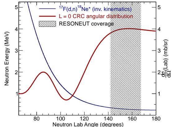
FIG. 1. Angular kinematics and angular distribution for an  $l = 0$  proton transfer for the  $^{17}\text{F}(d,n)^{18}\text{Ne}^*$  reaction in inverse kinematics, populating a state at 4.5 MeV excitation energy. The primary y-axis and the thin solid-line graph represent neutron-energy, the secondary y-axis and the thick solid-line graph represent the differential cross-section in the laboratory system, as predicted by a coupled reaction channel (CRC) calculation.
