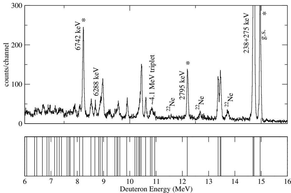
**Figure 2.** The top panel shows observed deuteron energy spectrum at  $29^\circ$  while the bottom panel shows the expected energies for the population of known levels in the  $^{20}\text{Ne}(p,d)^{19}\text{Ne}$  reaction at the same angle and a bombarding energy of 30 MeV. Peaks labeled with stars were used for energy calibration.
