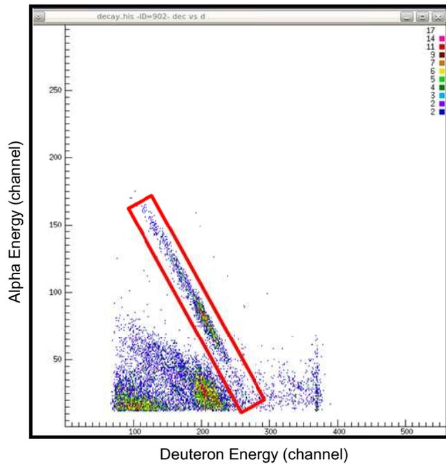
**Figure 3.** Decay energies plotted as a function of deuteron energies. Deuterons populating unbound  $^{19}\text{Ne}$  levels show the expected correlation with decay  $\alpha$  energies as indicated by the gate in this spectrum.
