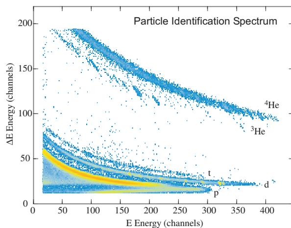
**Figure 1.** A particle identification spectrum from one of the SIDAR telescopes. The deuterons of interest are cleanly separated from other particle groups.
