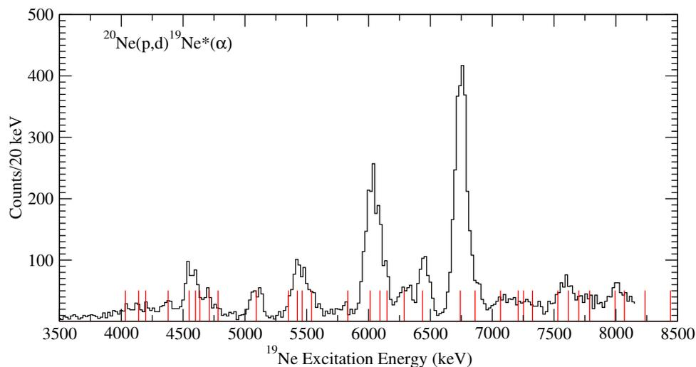
**Figure 4.** The deuteron energy spectrum in coincidence with decay  $\alpha$  particles. As expected, decay  $\alpha$  events are observed to start at the  $\alpha$  threshold except for random coincidences producing a continuous background. The vertical lines indicate the previously-measured  $^{19}\text{Ne}$  excitation energies. Small peaks are observed for the important 4.1-MeV triplet of states.
