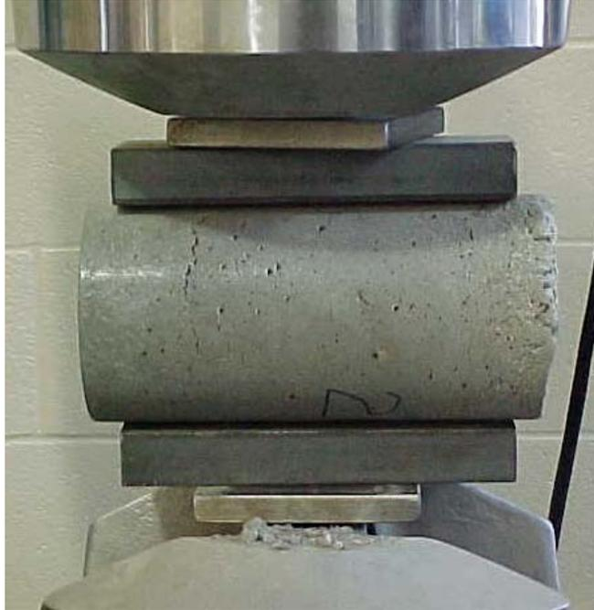
Figure 4: Split tensile strength testing of concrete.
