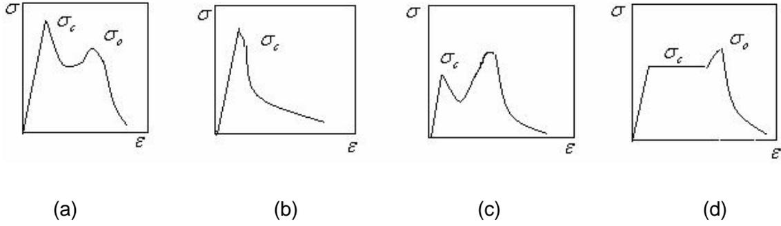
Figure 7: Failure modes of fiber reinforced concrete
