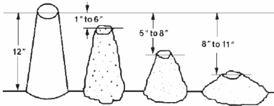
Figure 6: Comparison of typical slumps [<http://www.nrmca.org/aboutconcrete/cips/CIP%2022p.pdf>].
