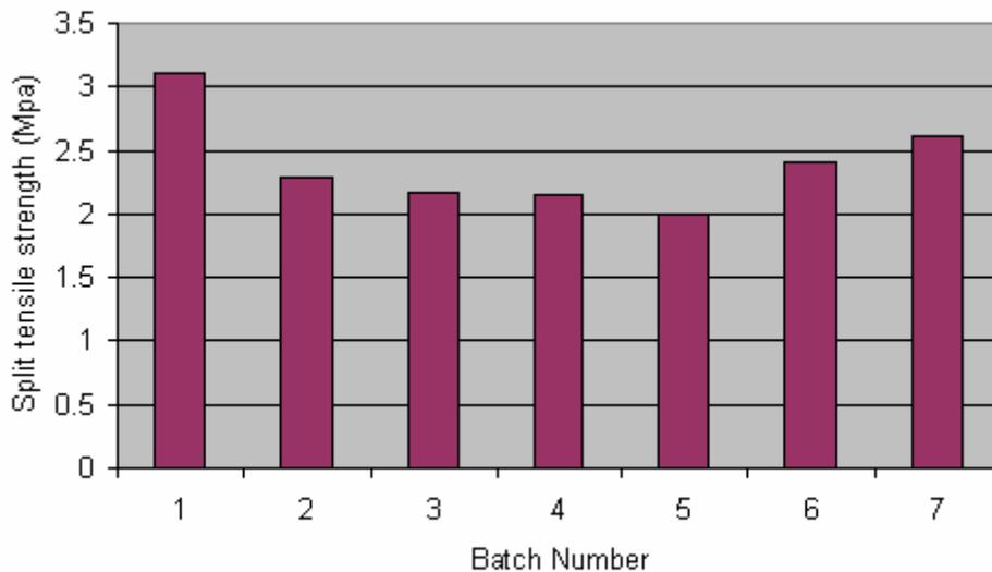
Figure 11: Variation of split tensile strength of concrete.
