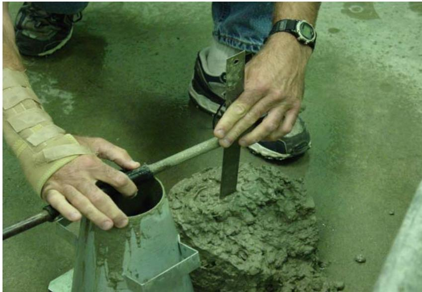
Figure 5: Slump testing concrete
