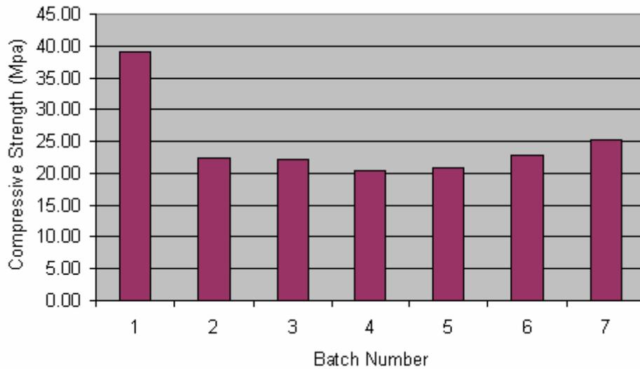
Figure 10. Variation of the compressive strength of concrete.
