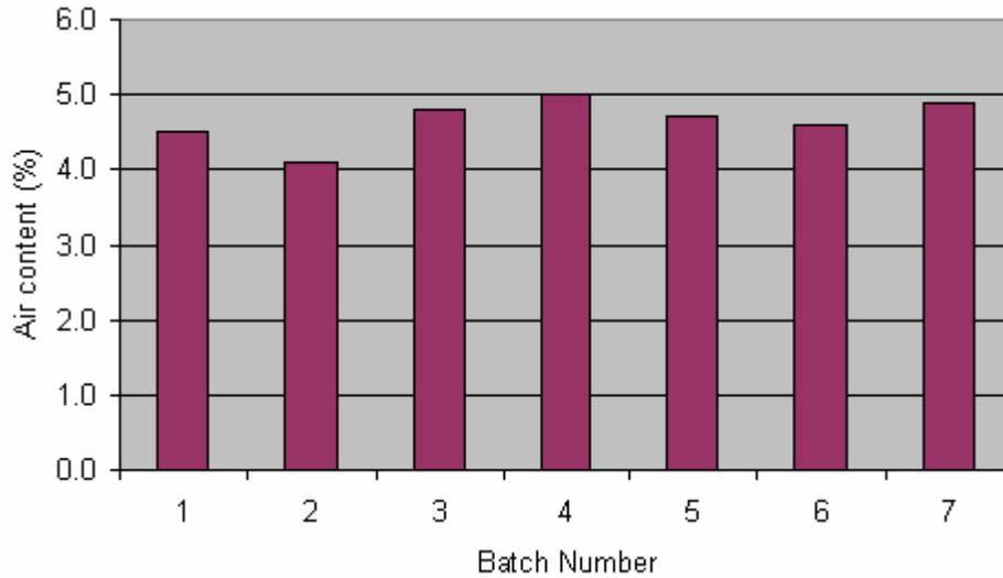
Figure 14: Results of air content for concrete.
