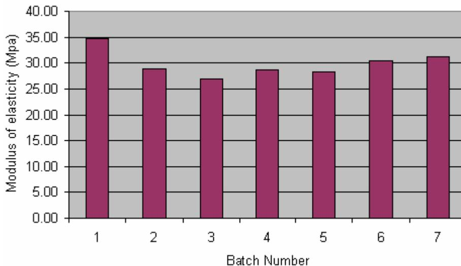
Figure 12: Variation of modulus of elasticity of concrete.
