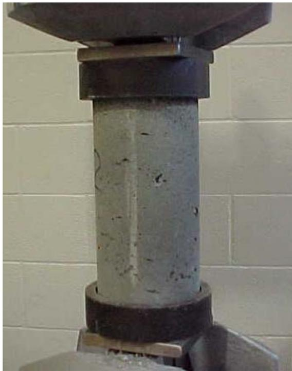
Figure 3: Concrete in compression test.
