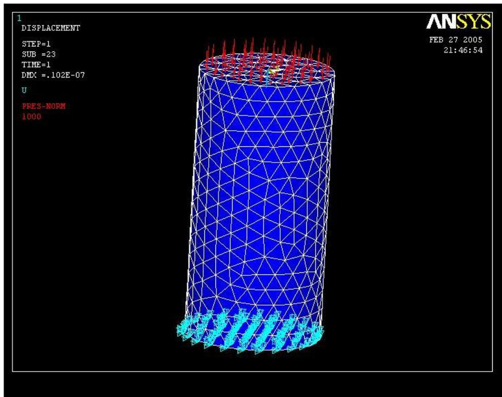
Figure 8: Constraints and load applied to model.
