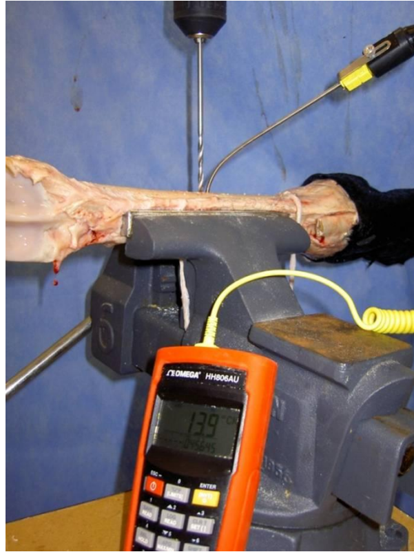
Figure 2.1. An equine third metatarsal bone in the testing device with thermocouples and the hand recorder in place
