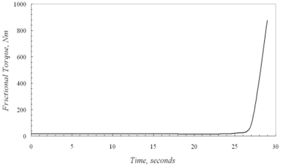
Figure 4.6 - Variation of frictional torque during start-up – Note that the frictional torque increased to 50 times the initial frictional torque to indicate seizure
