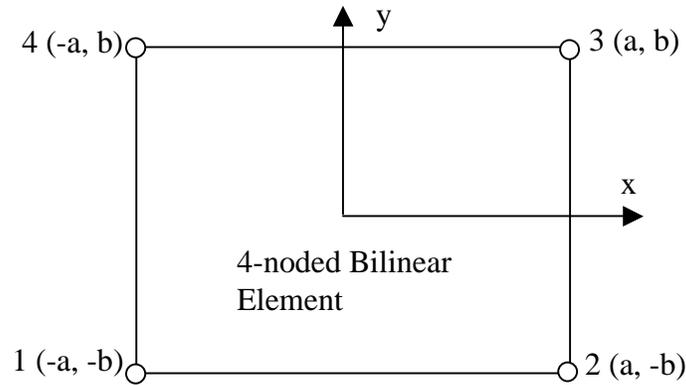
Figure 3.1 – 4-noded bilinear element
