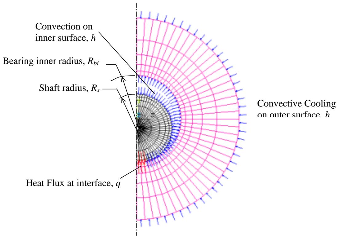
Figure 4.2 - Finite Element Model for Thermal Analysis, with loads and boundary conditions. (Not to scale)
