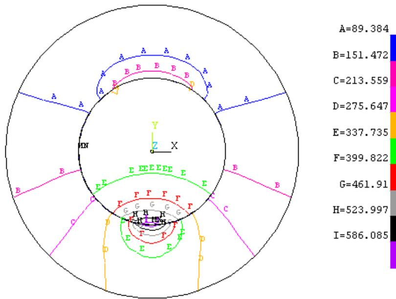
Figure 6.10 – Temperature contour 3 seconds after initialization of ovalization
