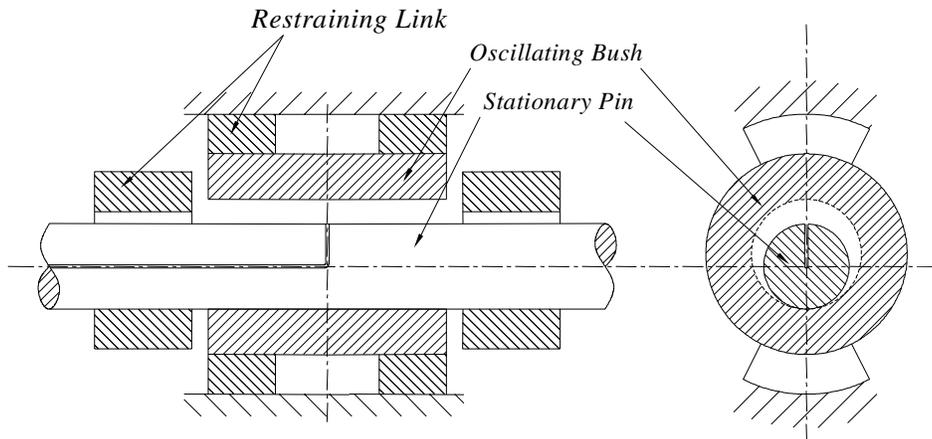
Figure 6.6 – Schematic of a Retention track assembly
