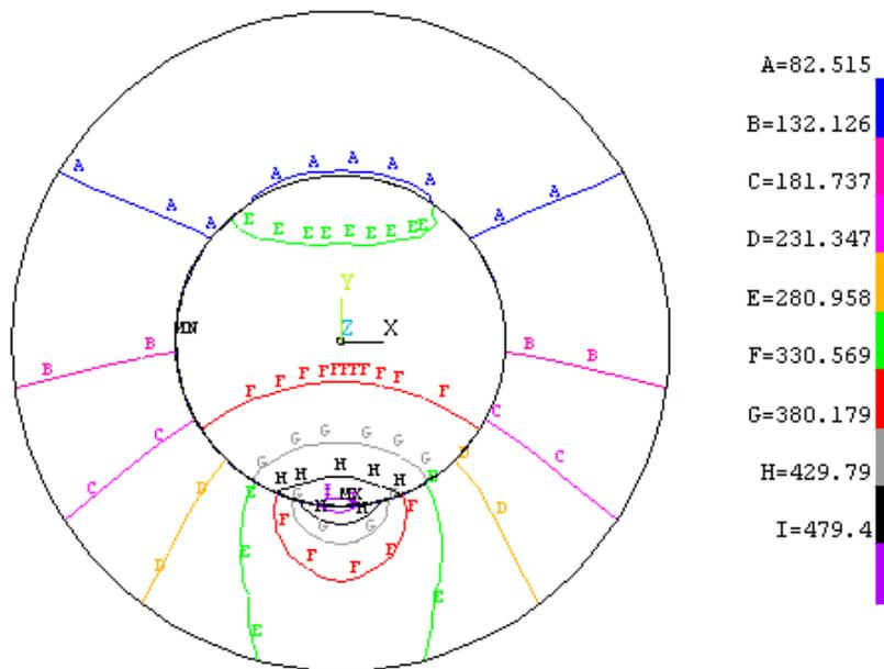
Figure 6.9 – Temperature contour 1 second after initialization of ovalization
