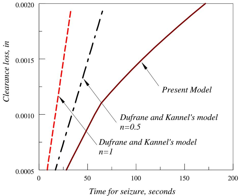
Figure 4.9 – Comparison of seizure time with Dufrane and Kannel's model and the present model. Note:  $n$  = heat partition factor
