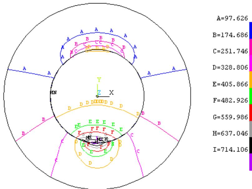
Figure 6.11 – Temperature contour 6 seconds after initialization of ovalization
