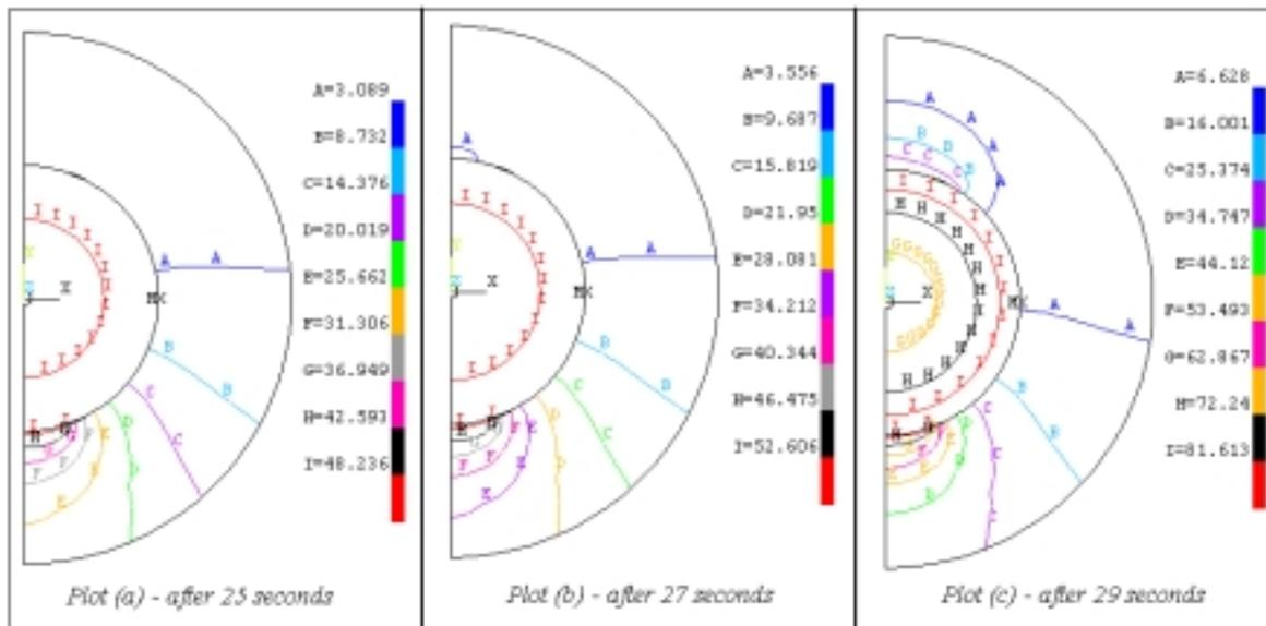
Figure 4.4 – Temperature rise as a function of time in a journal bearing during start up
