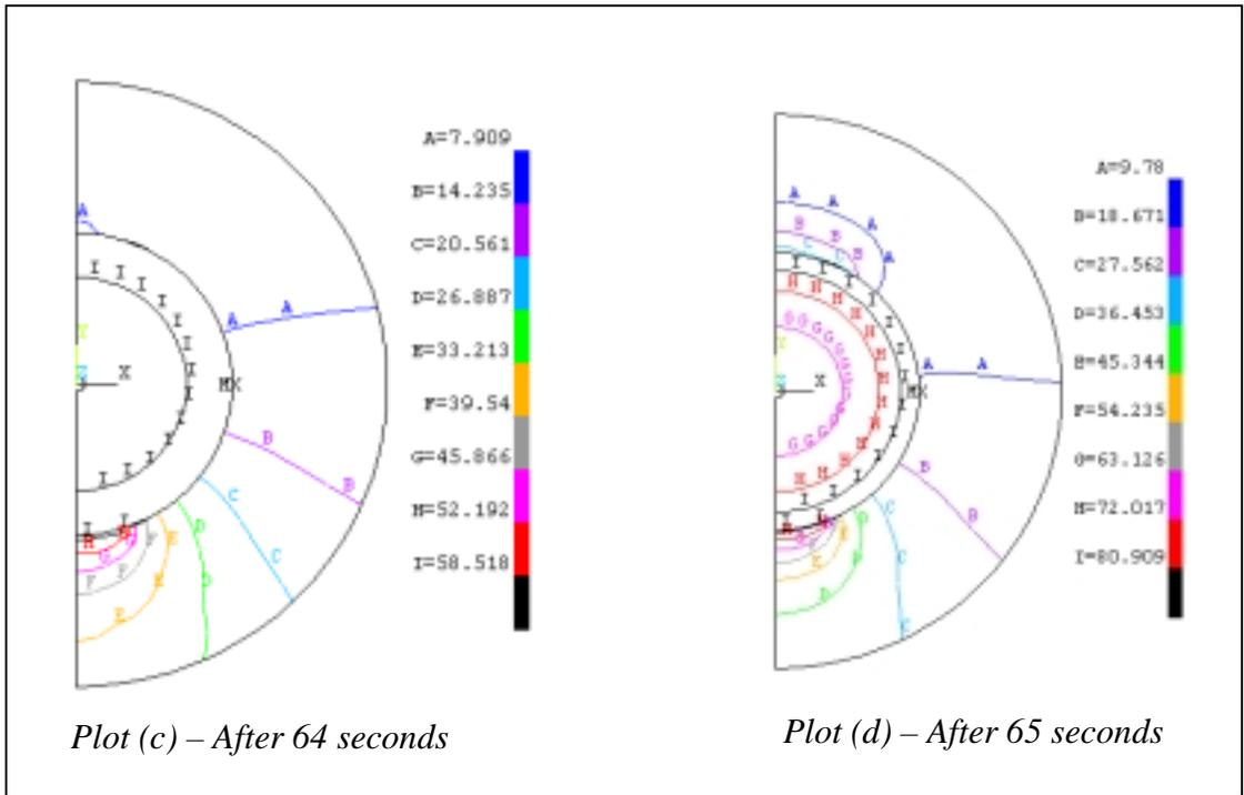
Figure 5.3c,d – Plots of temperature rise during a transient flow disturbance
