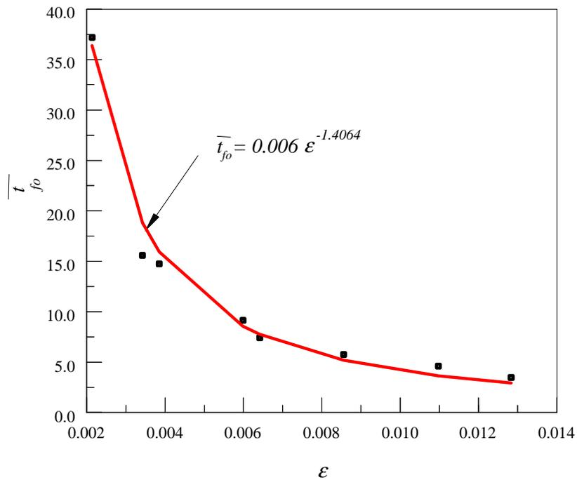
Figure 6.12 – Thermal Strain vs non-dimensional failure time
