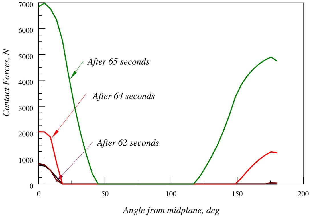
Figure 5.4 - Variation of contact force after the onset of ovalization due to flow disturbance
