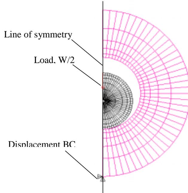
Figure 4.3 - ANSYS Model for Elastic Analysis, with loads and boundary conditions
