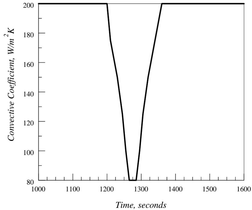
Figure 5.2 – Variation of convective HT coefficient during lubricant perturbation
