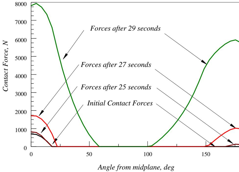
Figure 4.5 - Variation of contact forces with time during start-up
