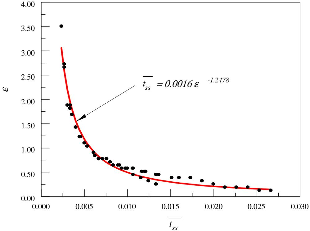
Figure 4.8 – Variation of non-dimensional seizure time with thermal strain
