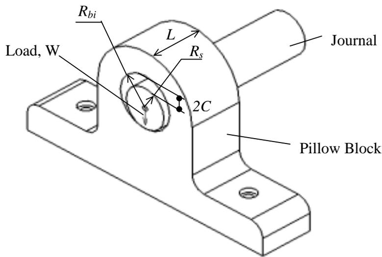
Figure 4.1 – Schematic of a journal supported on a pillow block
