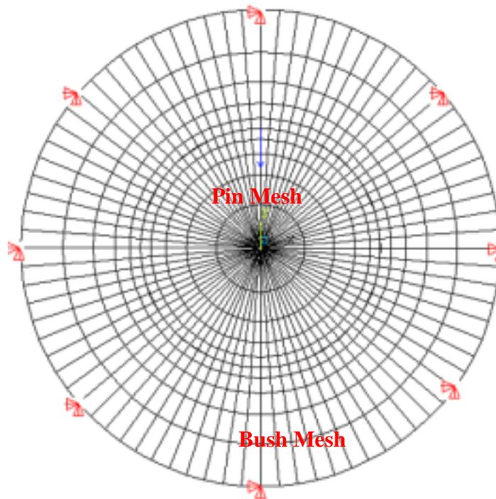
Figure 6.5 – Mesh pattern for the oscillating pin-bushing assembly
