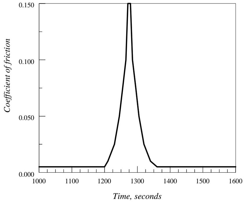
Figure 5.1 – Variation of friction coefficient during lubricant perturbation
