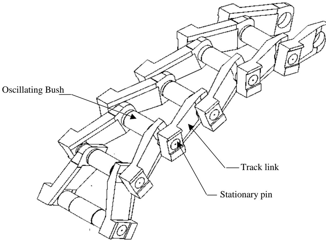
Figure 6.1 – Track Retention Assembly with the oscillating pin and bushing
