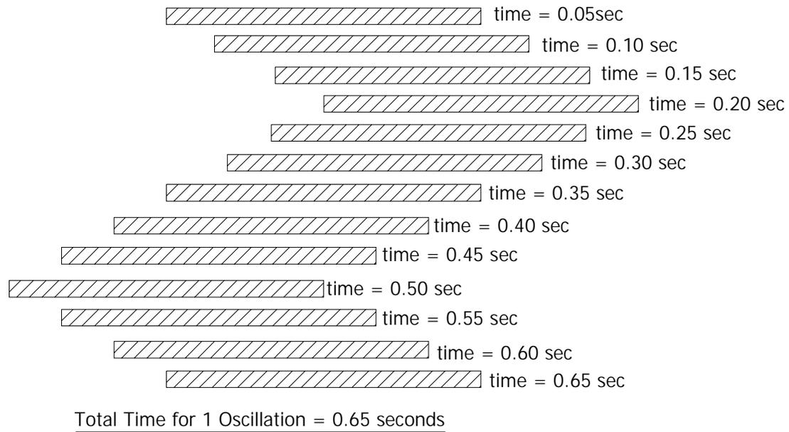
Figure 6.3 –Application of oscillating heat flux as a function of time and space
