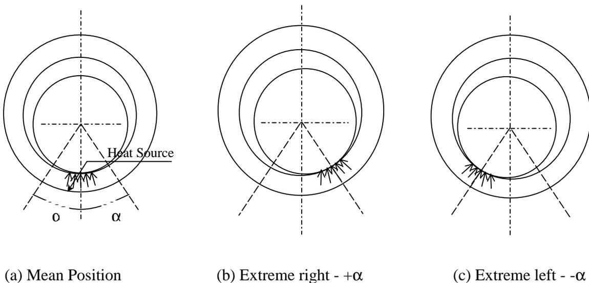
Figure 6.2 Schematic of application of oscillating flux,  $\alpha$  is the oscillation angle
