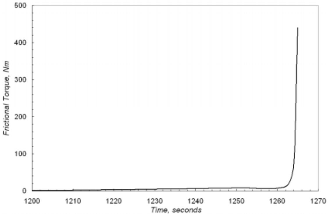
Figure 5.5 – Variation of frictional torque when a transient flow disturbance occurred
