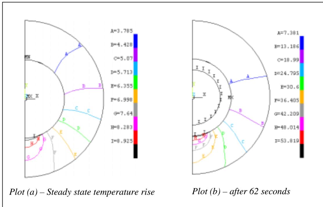
Figure 5.3a, b – Plots of temperature rise during a transient flow disturbance
