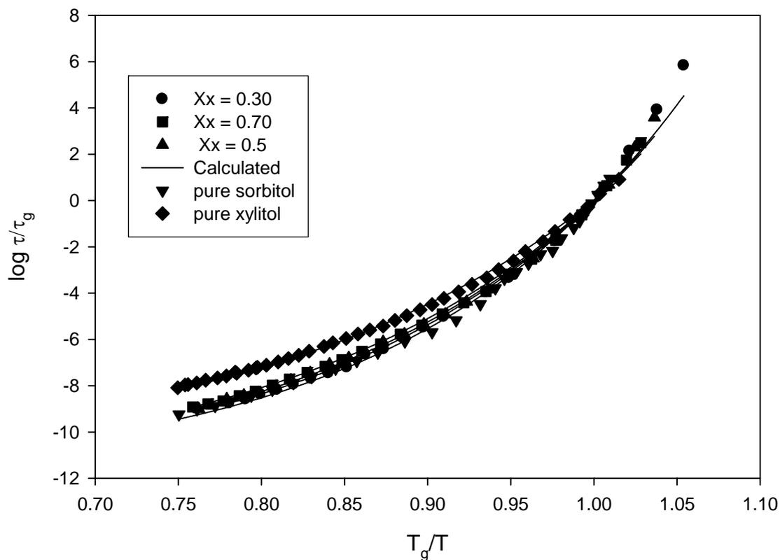
**Figure 17** Dielectric relaxation time versus temperature for sorbitol-xylitol mixtures and for pure sorbitol and xylitol. Experimental data are designated by symbols  $x_x = 0.0$  ( $\blacktriangledown$ ),  $x_x = 0.3$  ( $\bullet$ ),  $x_x = 0.5$  ( $\blacksquare$ ),  $x_x = 0.7$  ( $\blacktriangle$ ), and  $x_x = 1.0$  ( $\blacklozenge$ ), calculated values (and regression of pure sorbitol and xylitol data) by solid lines.
