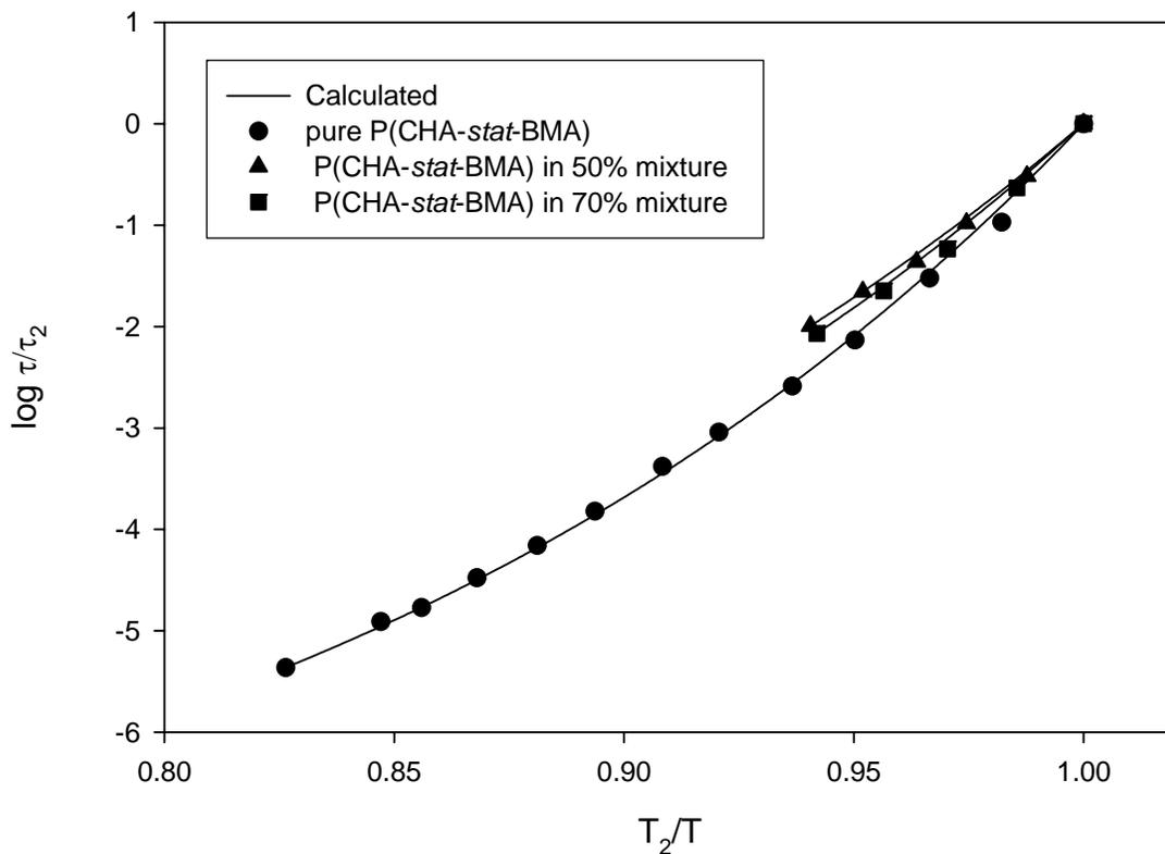
**Figure 23** Plot of temperature dependence of relaxation time showing experimental data for pure P(CHA-*stat*-BMA) (●), P(CHA-*stat*-BMA) relaxation in 50 wt% P(CHA-*stat*-BMA) and PS mixture (▲), and in 70 wt% P(CHA-*stat*-BMA) and PS mixture (■). Lines are fits of experimental data for pure P(CHA-*stat*-BMA), and calculated dielectric relaxation times for mixtures.
