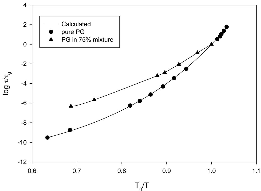
**Figure 30** Plot of temperature dependence of relaxation time showing experimental data for pure PG (●) and PG relaxation in 75 wt% aqueous PG solution (▲). Lines are fits of experimental data for pure PG, and calculated dielectric relaxation times for the solution.
