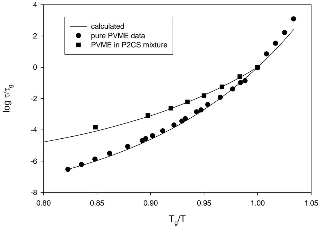
**Figure 22** Plot of temperature dependence of relaxation time showing experimental data for pure PVME (●) and PVME relaxation in a blend with P2CS (■). Solid lines are fits of experimental data for pure PVME, and calculated dielectric relaxation times for the blend.
