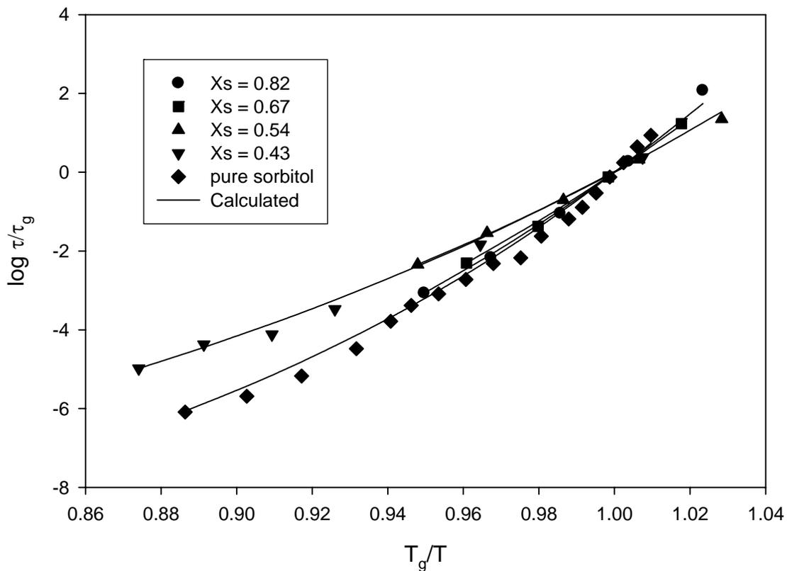
**Figure 15** Dielectric relaxation time versus scaled temperature for four sorbitol-glycerol mixtures and for pure sorbitol. Experimental data are designated by symbols,  $x_s = 1.0$  ( $\blacklozenge$ ),  $x_s = 0.82$  ( $\bullet$ ),  $x_s = 0.67$  ( $\blacksquare$ ),  $x_s = 0.54$  ( $\blacktriangle$ ) and  $x_s = 0.43$  ( $\blacktriangledown$ ), calculated values (and regression of pure sorbitol data) by solid lines.
