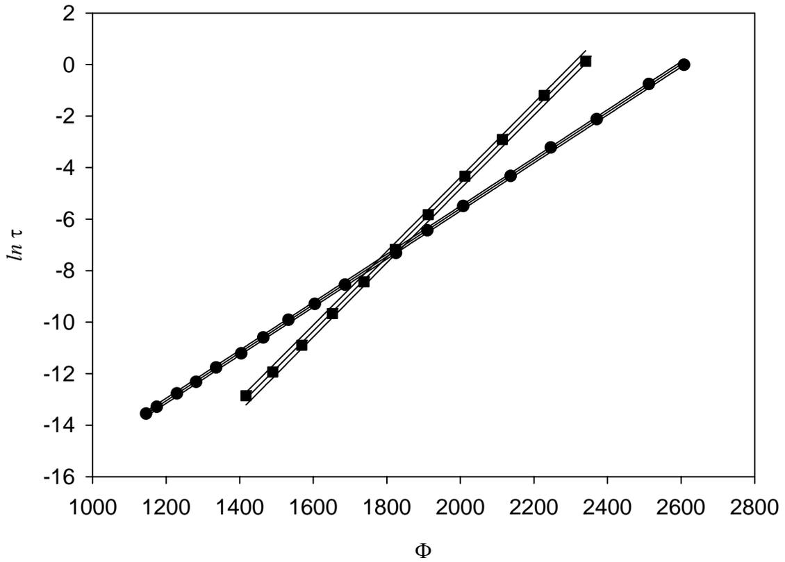
**Figure 13** Graph of  $\ln \tau$  vs.  $\Phi$  for PGEC at  $P = 95.5$  MPa (●) and at  $T = 293.5$  K (■). Lines indicate the predictions and their 95% prediction intervals.  $\Phi$  has been calculated using the value of parameter  $\nu$  given in Table 1 and the parameter  $h = 2.94 \times 10^{-20}$  J.
