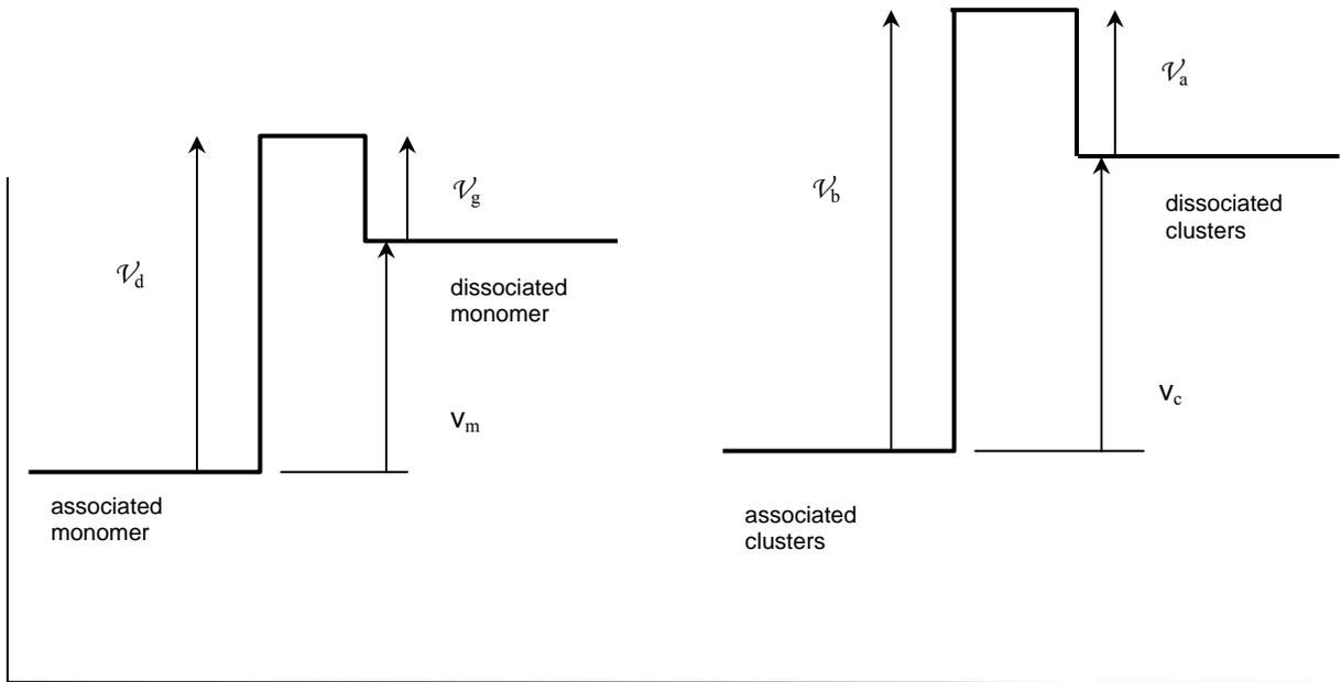
**Figure 4** Elements of the energy landscape. Energy and volume barriers are based on transition state theory for reversible monomer–cluster growth and dissociation and cluster–cluster association and breakage [Eqs. (17) and (18)]. Energies and volumes of transformation are differences in activation energies and volumes:  $h_m = E_d - E_g$ ,  $h_c = E_b - E_a$ ,  $v_m = \mathcal{V}_d - \mathcal{V}_g$ , and  $v_c = \mathcal{V}_b - \mathcal{V}_a$ .
