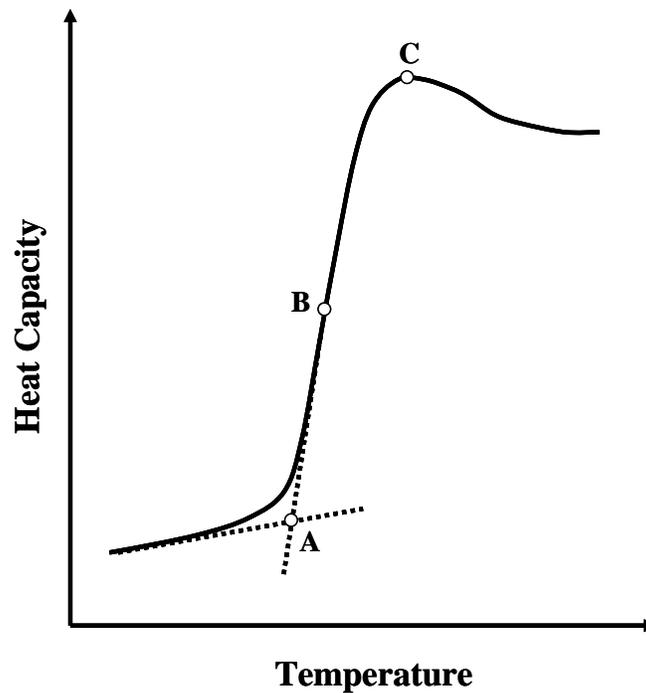
**Figure 2** Plot of heat capacity versus temperature resulting from differential scanning calorimetry. Point A (the intersection of lines drawn through the two straight portions of the plot) is normally used to represent the calorimetric glass transition temperature, although points C (the maximum in the plot) and B (average of the methods for points A and C) are also found in the literature<sup>11</sup>.
