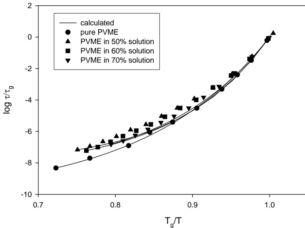
**Figure 24** Plot of temperature dependence of relaxation time showing experimental data for pure PVME ( $\bullet$ ), PVME relaxation in 50 wt% PVME toluene solution ( $\blacktriangle$ ), PVME relaxation in 60 wt% PVME toluene solution ( $\blacksquare$ ), and PVME relaxation in 70 wt% PVME toluene solution. Lines are fits of experimental data for pure PVME, and calculated dielectric relaxation times for solutions.
