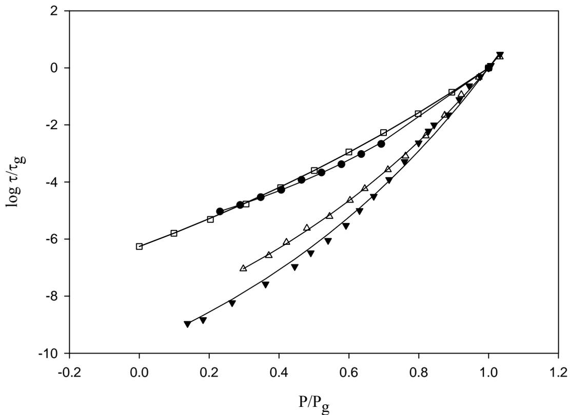
**Figure 7** Plot of the log of scaled dielectric relaxation time versus scaled pressure for PMTS ( $\square$ ), PPG ( $\triangle$ ), DGEB( $\bullet$ ) and DEP ( $\blacktriangledown$ ) at  $\sim 293$  K. Model fits are shown as lines with parameters of Table 1 and experimental data<sup>27,25,92,93</sup> as points. The defined point at  $\log \tau_i^*/\tau_g = 0$  at  $P/P_g = 1$  has been added to the data sets.
