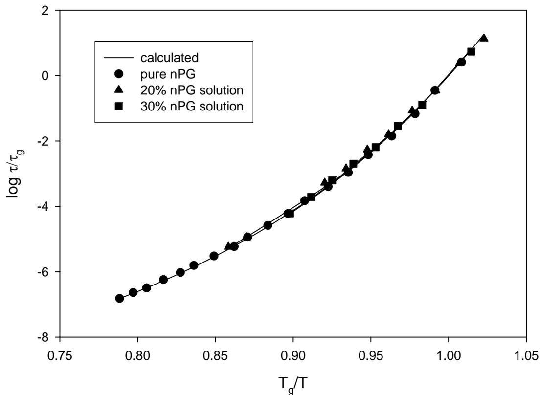
**Figure 26** Plot of temperature dependence of relaxation time showing experimental data for pure *nPG* (●), *nPG* relaxation in 20 wt% aqueous *nPG* solution (▲), and *nPG* relaxation in 30 wt% aqueous *nPG* solution (■). Lines are fits of experimental data for pure *nPG*, and calculated dielectric relaxation times for solutions.
