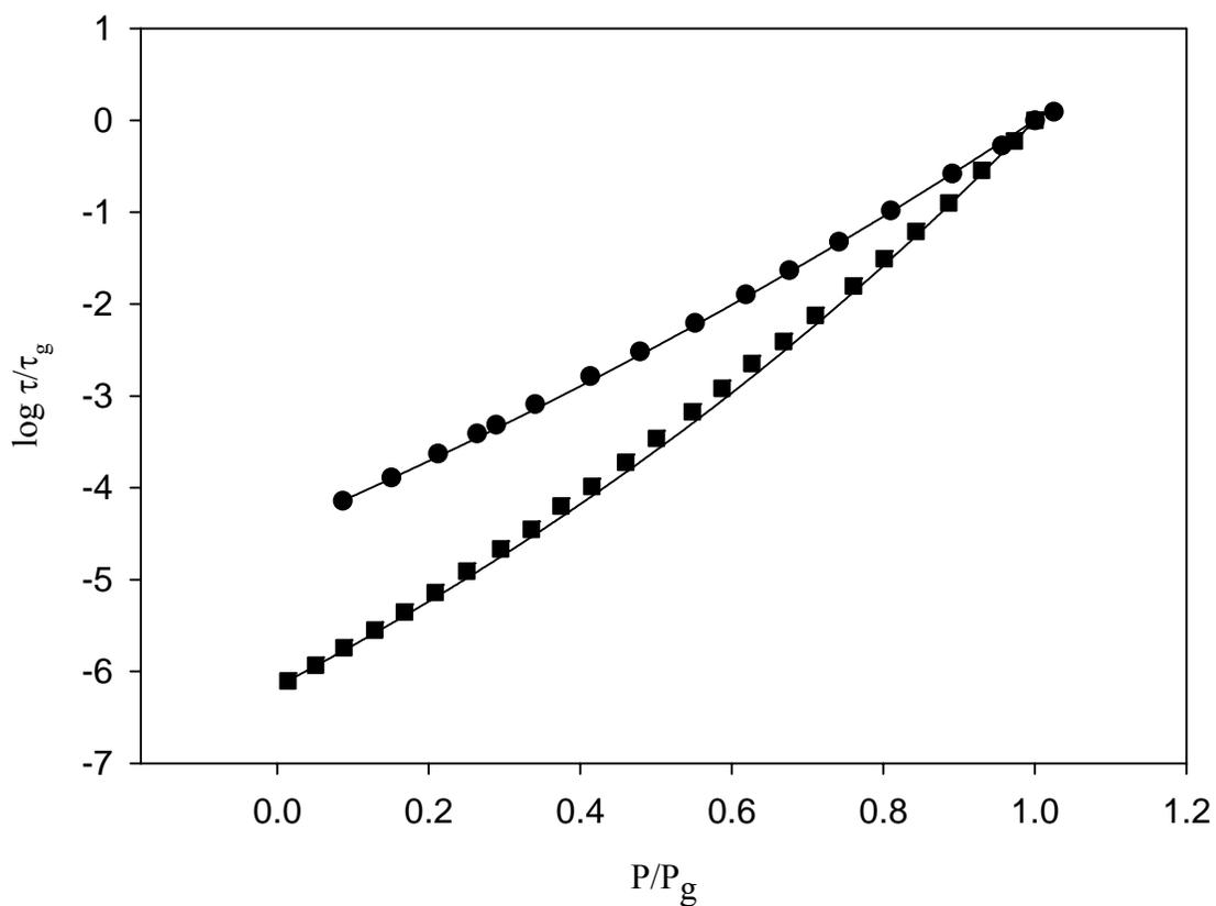
**Figure 11** Predicted  $\log \tau/\tau_g$  for PMPS vs. experimental data at  $T = 263$  K (●) and  $T = 273$  K (■). The lines represent the prediction with the parameter  $\nu = 2.48 \times 10^{-29} \text{ m}^3$ . The defined point at  $\log \tau/\tau_g = 0$  at  $P/P_g = 1$  has been added to the data sets.
