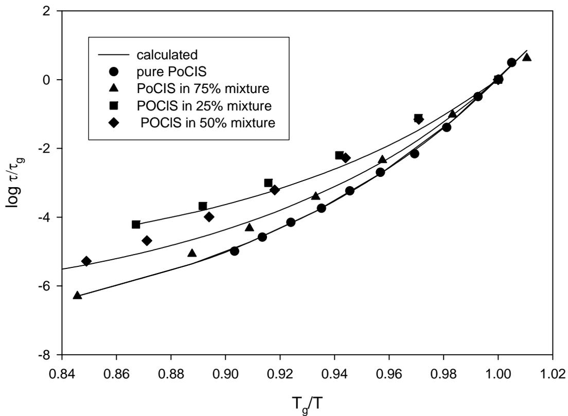
**Figure 19** Plot of temperature dependence of relaxation time showing experimental data for pure PoCIS ( $\bullet$ ), PoCIS relaxation in 25wt% PoCIS and PS mixture ( $\blacksquare$ ), in 50wt% PoCIS and PS mixture ( $\blacklozenge$ ), and in 75 wt% PoCIS and PS mixture ( $\blacktriangle$ ). Lines are fits of experimental data for pure PoCIS, and calculated dielectric relaxation times for mixtures.
