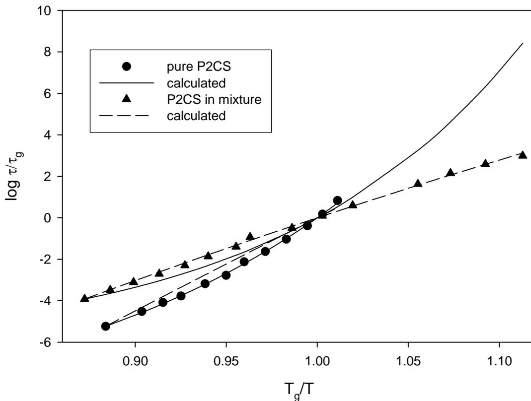
**Figure 21** Plot of temperature dependence of relaxation time showing experimental data for pure P2CS (●) and P2CS relaxation in a mixture with PVME (▲). Solid lines are fits of experimental data for pure P2CS, and calculated dielectric relaxation for the mixture. Dashed lines are fits of experimental data for P2CS in the blend, and calculated dielectric relaxation times for pure P2CS.
