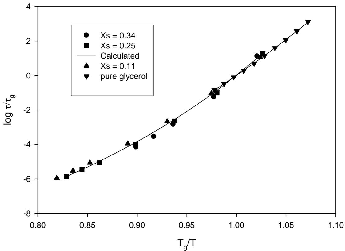
**Figure 16** Dielectric relaxation time versus scaled temperature for three sorbitol-glycerol mixtures and for pure glycerol. Experimental data are designated by symbols,  $x_s = 0.34$  (●),  $x_s = 0.25$  (■),  $x_s = 0.11$  (▲), and  $x_s = 0.0$  (▼), calculated values (and regression of pure glycerol data) by solid lines.
