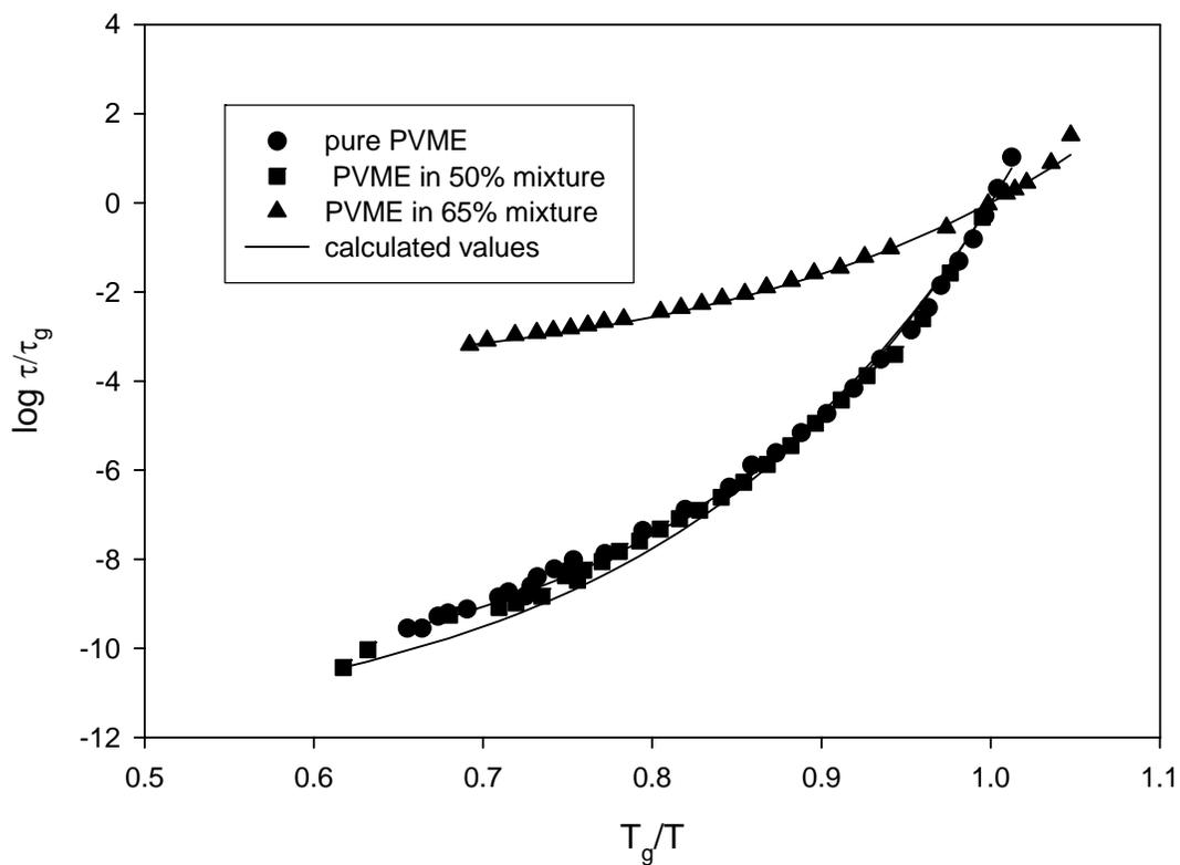
**Figure 20** Plot of temperature dependence of relaxation time showing experimental data for pure PVME (●) PVME relaxation in 50 wt% PVME and PS mixture (■), and PVME relaxation in 65 wt% PVME and PS mixture (▲). Solid lines are fits of experimental data for pure PVME, and calculated dielectric relaxation times for mixtures.
