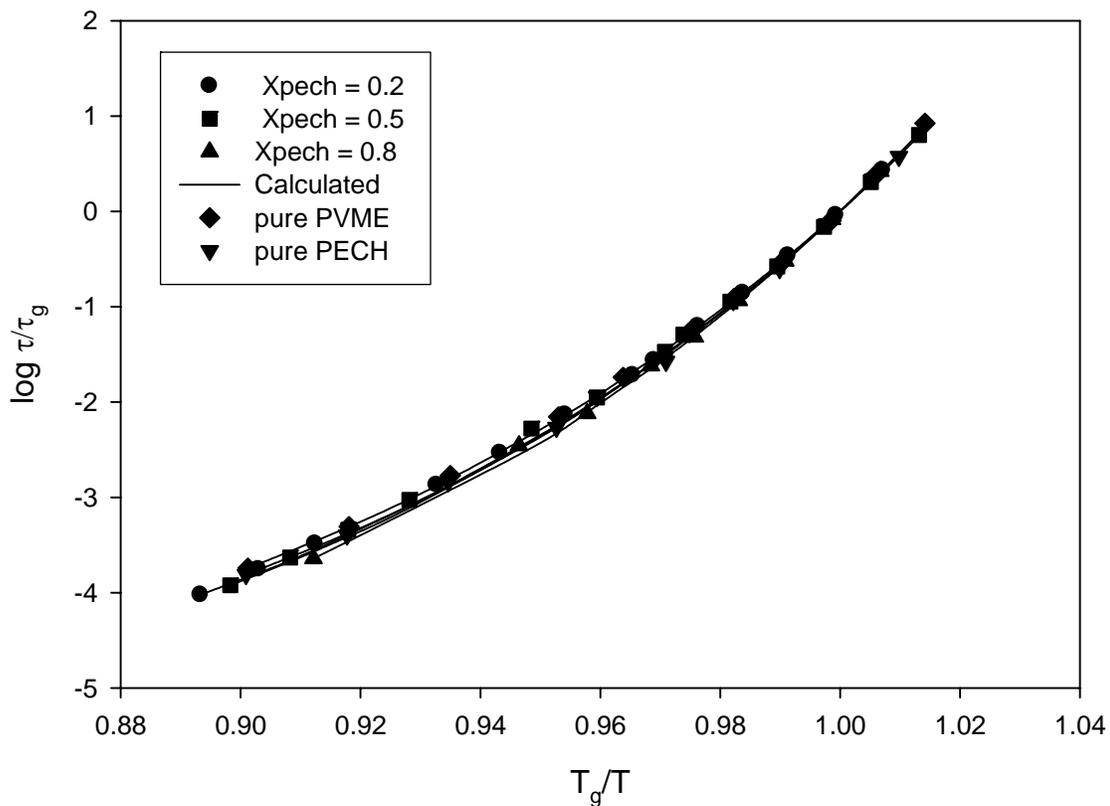
**Figure 18** Dielectric relaxation time versus temperature for PECH-PVME mixtures and for pure PECH and PVME. Experimental data are designated by symbols  $x_{PECH} = 0.0$  (▼),  $x_{PECH} = 0.2$  (●),  $x_{PECH} = 0.5$  (■),  $x_{PECH} = 0.8$  (▲), and  $x_{PECH} = 1.0$  (◆), calculated values (and regression of pure PECH and PVME data) by solid lines.
