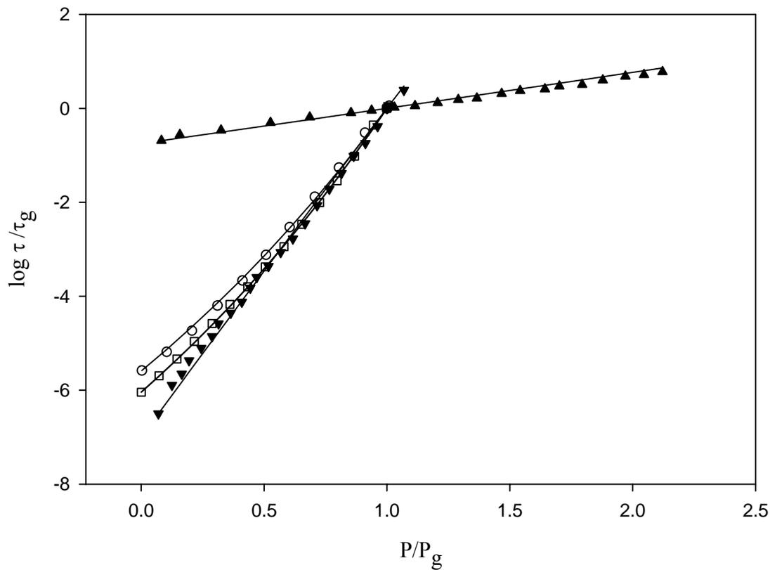
**Figure 6** Plot of the log of scaled dielectric relaxation time versus scaled pressure for PBD ( $\square$ ), IPCB ( $\blacktriangle$ ), PGEC ( $\circ$ ) and DAR ( $\blacktriangledown$ ) at  $\sim 293$  K. Model fits are shown as lines with parameters of Table 1 and experimental data <sup>15, 90, 91, 94</sup> as points. The defined point at  $\log \tau_{f^*} / \tau_g = 0$  at  $P/P_g = 1$  has been added to the data sets.
