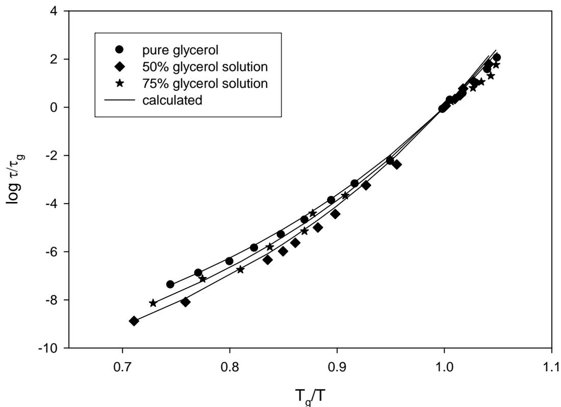
**Figure 29** Plot of temperature dependence of relaxation time showing experimental data for pure glycerol (●), glycerol relaxation in 50 wt% aqueous glycerol solution (◆), and glycerol relaxation in 75 wt% aqueous glycerol solution (★). Lines are fits of experimental data for pure glycerol, and calculated dielectric relaxation times for solutions.
