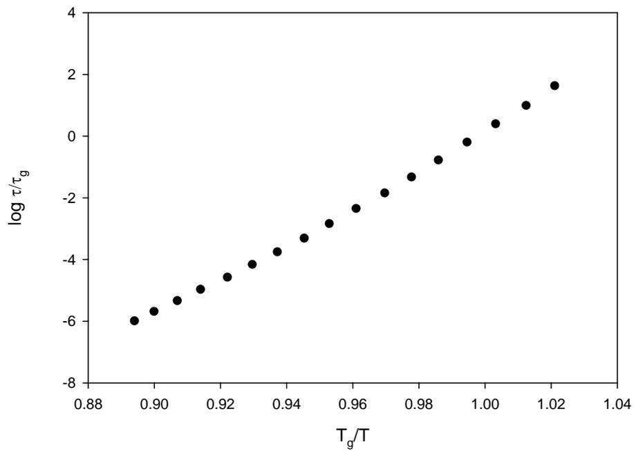
**Figure 3** Fragility plot for salol<sup>16</sup>, of scaled dielectric relaxation vs. scaled inverse temperature.
