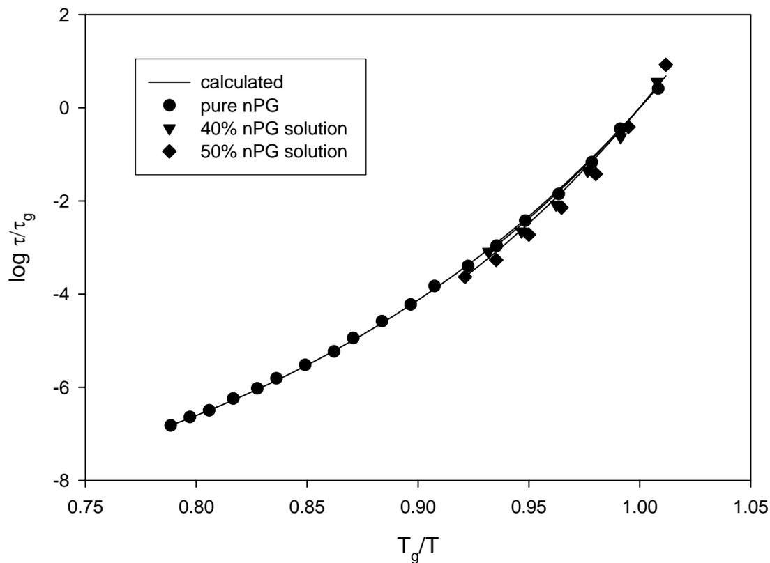
**Figure 27** Plot of temperature dependence of relaxation time showing experimental data for pure *nPG* (●), *nPG* relaxation in 40 wt% aqueous *nPG* solution (▼), and *nPG* relaxation in 50 wt% *nPG* solution (◆). Lines are fits of experimental data for pure *nPG*, and calculated dielectric relaxation times for solutions.
