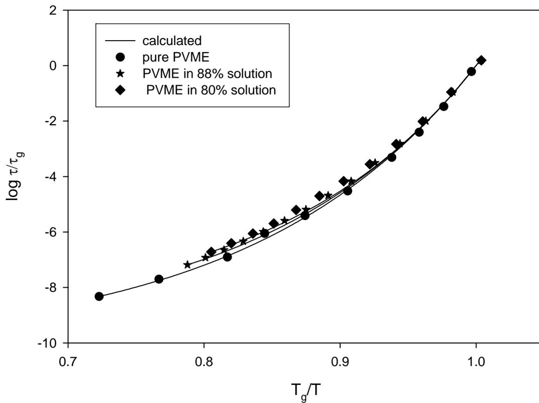
**Figure 25** Plot of temperature dependence of relaxation time showing experimental data for pure PVME (●), PVME relaxation in 80 wt% PVME toluene solution (◆), and PVME relaxation in 88 wt% PVME toluene solution (★). Lines are fits of experimental data for pure PVME, and calculated dielectric relaxation times for solutions.
