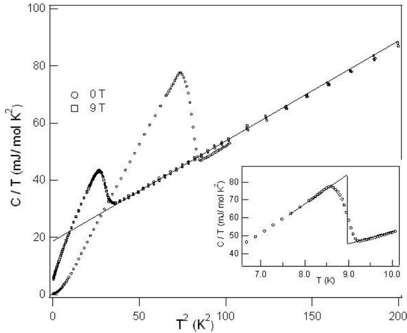
Figure 9. Characterization of  $\text{Mo}_3\text{Al}_2\text{C}$  by the measurement of specific heat at 0 and 9 T. Inset:  $C/T$  vs.  $T$  plot to determine the specific heat jump at the superconducting transition.
