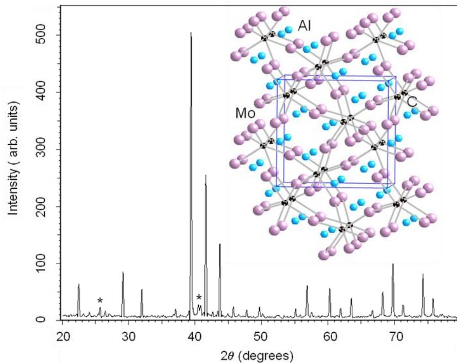
Figure 1. Powder X-ray diffraction pattern and schematic view of the crystal structure of polycrystalline  $\text{Mo}_3\text{Al}_2\text{C}$ . The \*'s in the figure indicate impurity peaks associated with elemental Mo and  $\text{Mo}_3\text{Al}_8$ .
