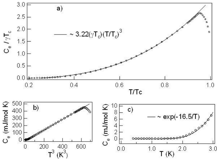
Figure 10. a) Superconducting electronic specific heat capacity ( $C_{es}$ ) vs. reduced temperature ( $T/T_c$ ) of  $\text{Mo}_3\text{Al}_2\text{C}$ . b)  $C_{es}$  vs.  $T^3$  plot and c)  $C_{es}$  vs.  $T$  at low temperature.
