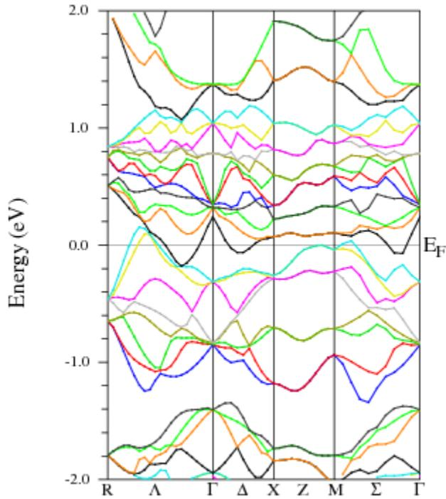
Figure 2. Section of the calculated electronic band structure along high symmetry directions for  $\text{Mo}_3\text{Al}_2\text{C}$  in the range of  $\pm 2$  around the Fermi energy  $E_F$ . The band structure is without spin-orbit coupling.
