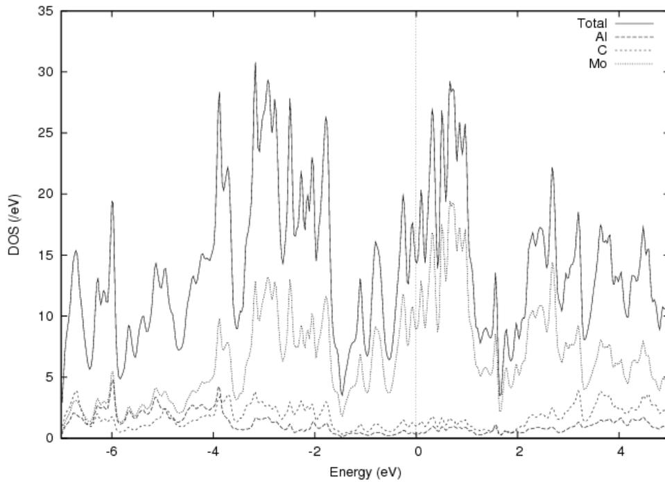
Figure 3. Section of total and atom-projected density of states (DOS; in states  $\text{eV}^{-1}$ ) for  $\text{Mo}_3\text{Al}_2\text{C}$  in the energy range  $-7$  to  $+5$  around the Fermi energy  $E_F$ . Energy scale is defined relative to  $E_F$ . The DOS is shown for scalar relativistic calculation only.
