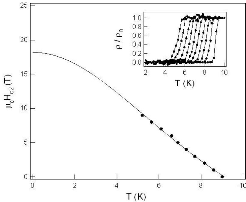
Figure 8. Upper critical field of  $\text{Mo}_3\text{Al}_2\text{C}$  as a function of temperature. The solid line is fit to Ginzburg-Landau theory (see text for details). Inset: Characterization of the superconducting transition under magnetic fields 0 T to 9 T from right to left.
