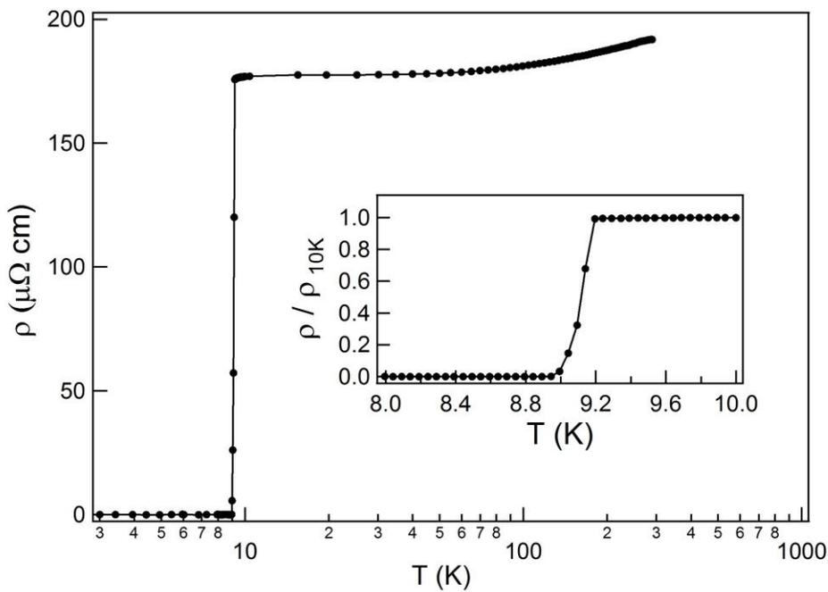
Figure 5. Semi-log plot of the resistivity of polycrystalline  $\text{Mo}_3\text{Al}_2\text{C}$  over the range of temperature from 3 to 290 K. The inset shows the superconducting transition at low temperature. The solid lines in both figures are a guide to the eye.
