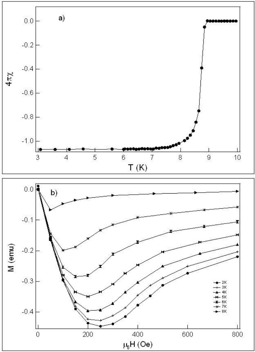
Figure 6. a) ZFC magnetic susceptibility measured at constant magnetic field of 30 Oe. b) Magnetization data with applied magnetic field at various temperatures.
