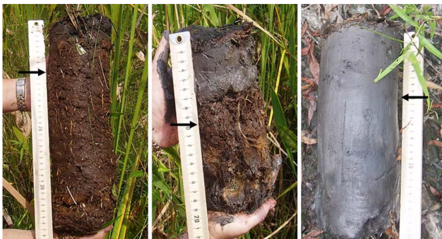
Fig. 4 Cores taken from the reference marsh (left), the marsh surrounding the southern canal (center), and the former spoil area of the southern canal which supports spoil vegetation (right). The arrows point to the 10 cm mark on each core
