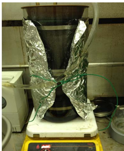
Figure 2.4 Reflux Used to Extract Asphalt
