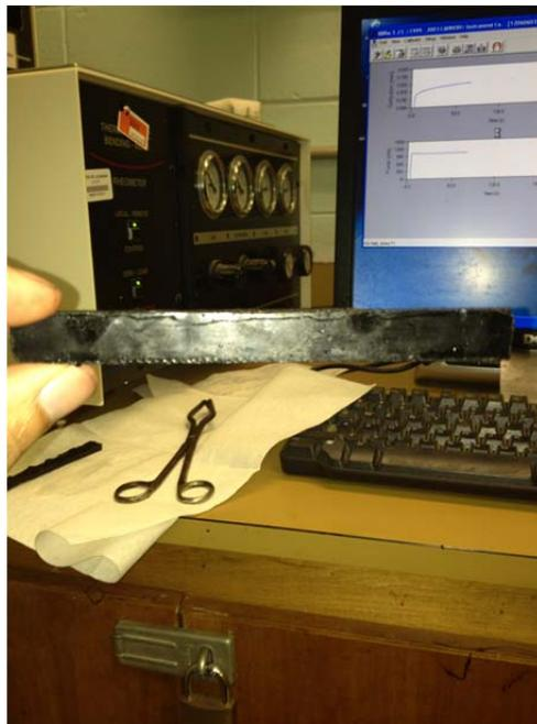
Figure 2.8 Bending Beam Rheometer
