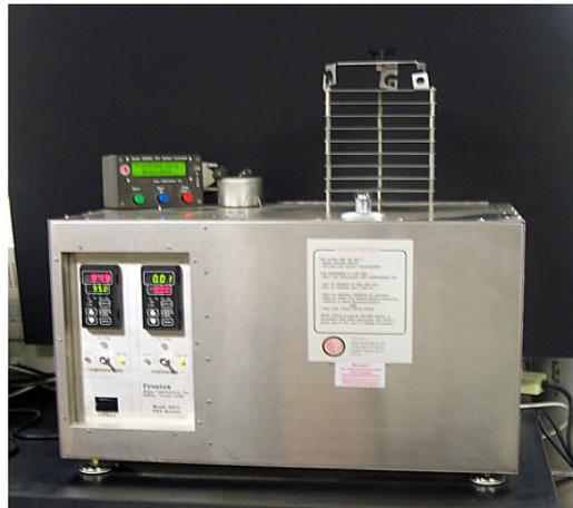
Figure 2.9 Pressure Aging Vessel (Obtained from [www.pavementinteractive.org](http://www.pavementinteractive.org))
