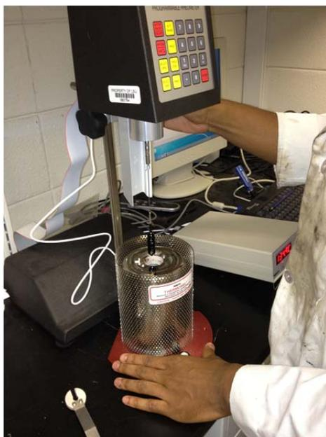
Figure 2.10 Rotational Viscometer
