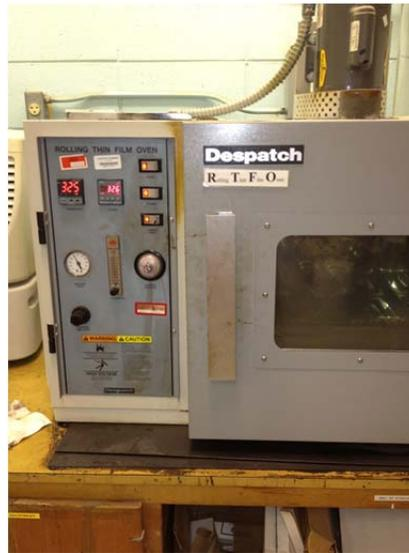
Figure 2.7 Rolling Thin Film Oven
