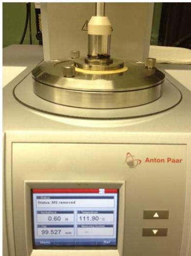
Figure 2.6 Dynamic Shear Rheometer
