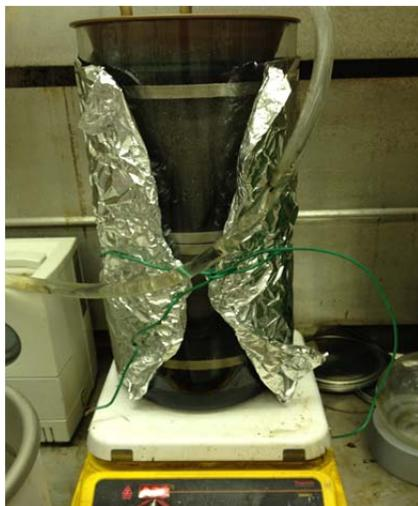
Figure 2.4 Reflux Used to Extract Asphalt
