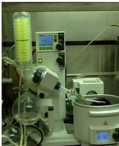
Figure 2.5 Rotovapor used to extract asphalt from TCE
