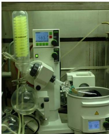
Figure 2.5 Rotovapor used to extract asphalt from TCE
