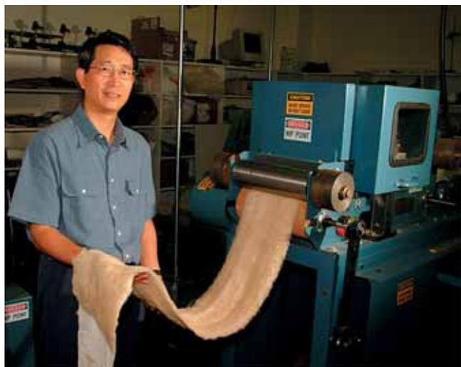
*Yan Chen holds the fiber web that has been needle-punched for further compaction.*
