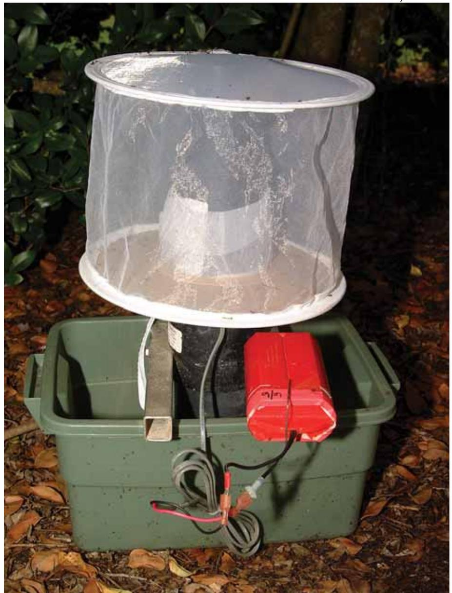
Figure 3: The CDC (for Centers for Disease Control) miniature light trap is typically hung from a tree and includes a light to attract flying mosquitoes and a fan to suck them into the white net tube. The cooler hanging next to the trap contains dry ice, which is carbon dioxide (CO<sub>2</sub>) in a solid state. CO<sub>2</sub> attracts mosquitoes.
