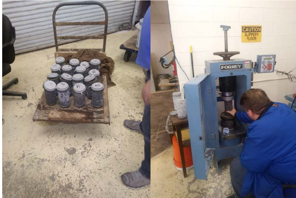
Figure 3. Ready for testing samples on the left and installation of the sample into the hydraulic press on the right.
