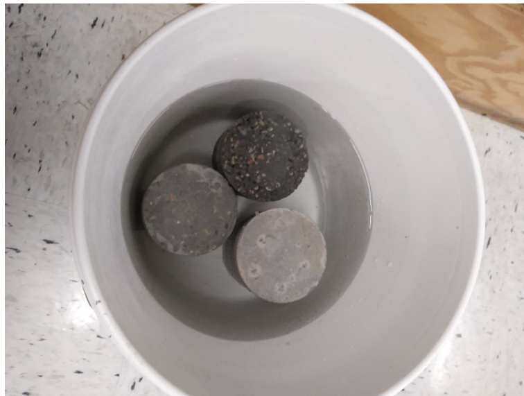
Figure 1. Water absorption test.
