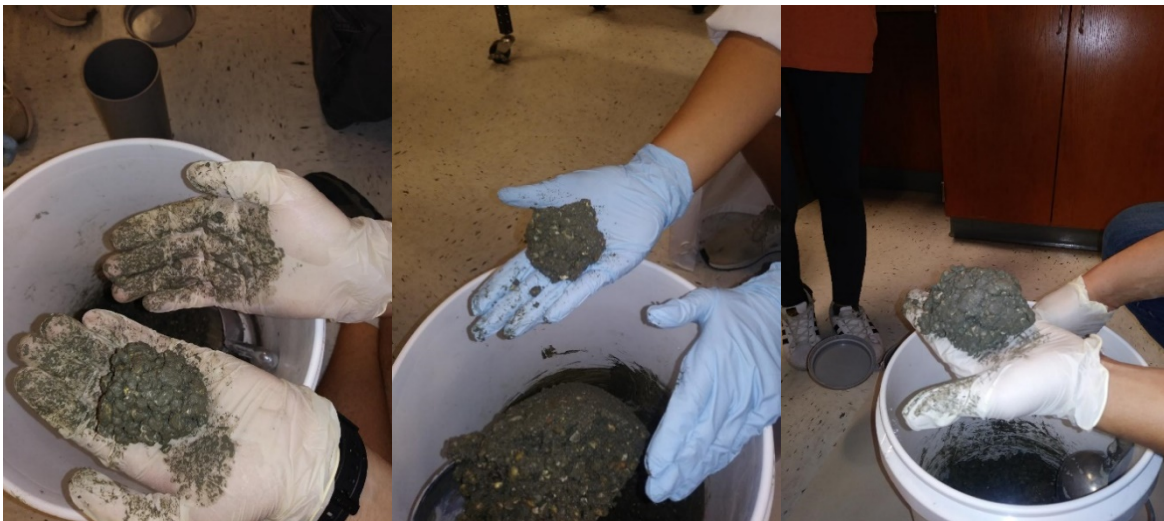
Figure 4. The ball test was performed in order to track water content in the mixture.
