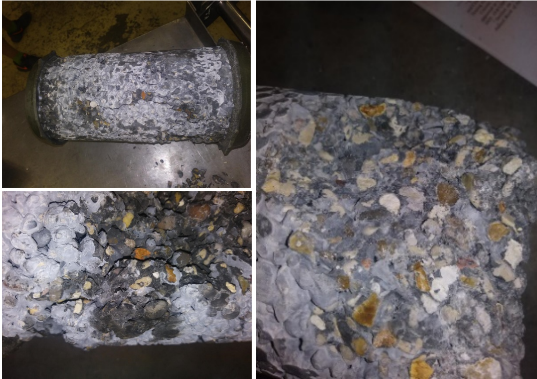
Figure 6. The crack is running from the top to the bottom of the sample cylinder (upper left picture). The piece of sample is missing due to compression test and the aggregate particles cut by crack (bottom left and right pictures).
