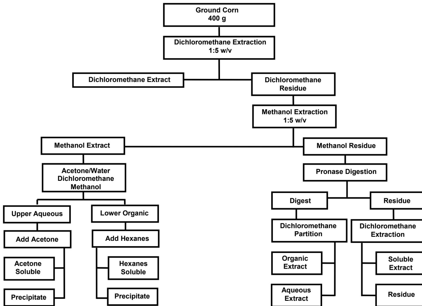
Figure 3.2. Flow diagram of the separation of AFB<sub>1</sub>-related decontamination by-products in corn following ozone treatment.
