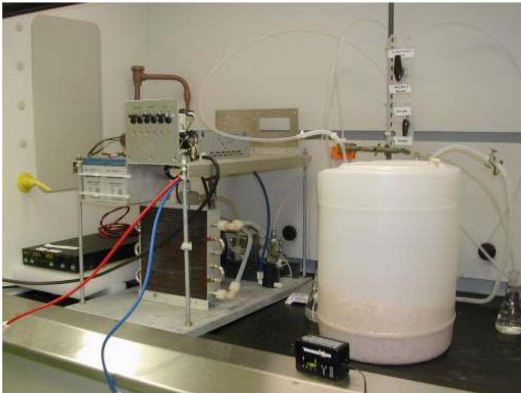
Figure 3.1. Set-up of the ozonation process.
