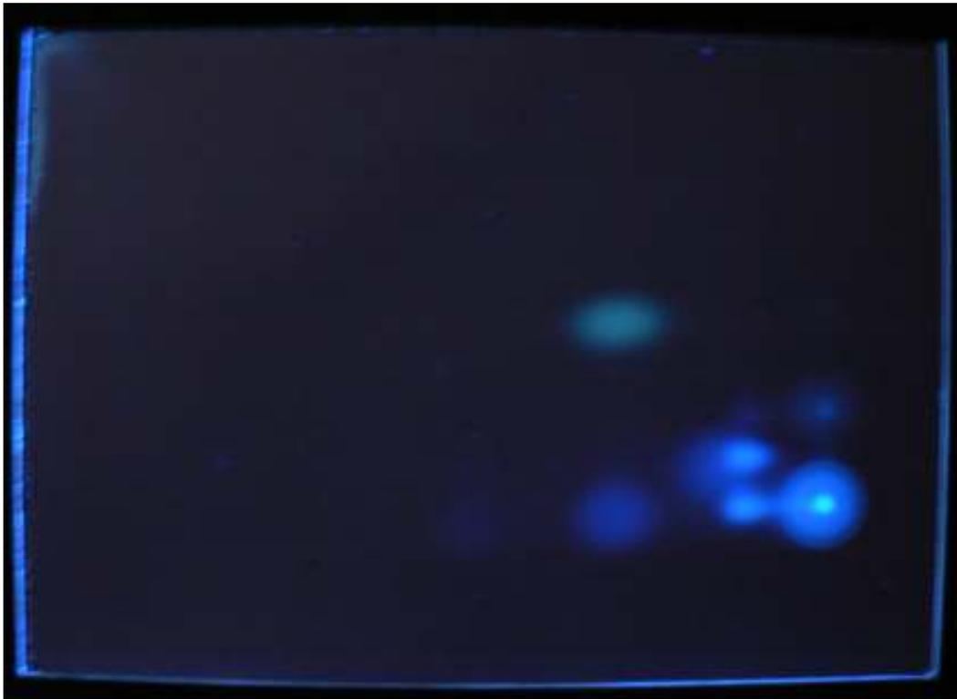
Figure 4.9. Two-dimensional TLC chromatogram of 60-sec ozonated standard AFB<sub>1</sub> developed first with ether+methanol+water (96:3:1) from right to left and with chloroform+methanol (9:1) from bottom to top.
