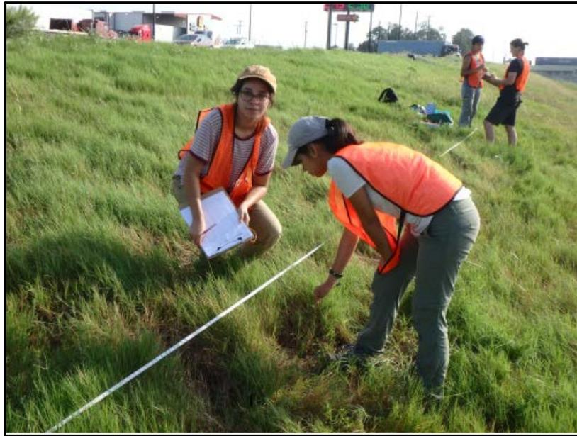
Figure 2. UTSA students measuring vegetation coverage along IH-35 using the line transect method.
