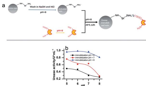
Fig. 1 (a) Scheme of urease immobilization processes. (b) The activity of the immobilized enzyme in buffer solution of different pHs. [(NH<sub>4</sub>)<sub>2</sub>SO<sub>4</sub>] = 0.1 M; [H<sub>2</sub>SO<sub>4</sub>] = 1 M; [urea] = 0.5 M; [urease]<sub>free</sub> = [urease]<sub>IM</sub> = 4 U mL<sup>-1</sup>.
