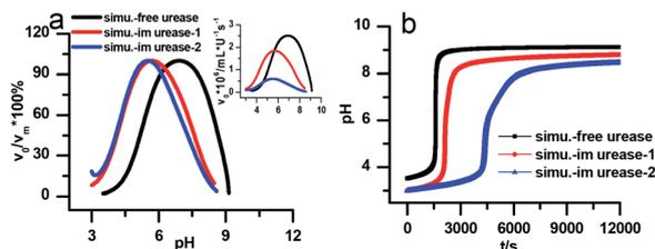
Fig. 7 Simulated kinetic profiles in the urea-urease- $H^+$  reaction. (a) The bell-shaped rate-pH curve is the larger graph with the relative value that are normalized to the maximum, the inset is the absolute rate data. (b) Clock reaction curves in the free and immobilized urease system. Parameters employed for each curve are listed in Table 1. Other fixed parameters value can be found in ESI.†
