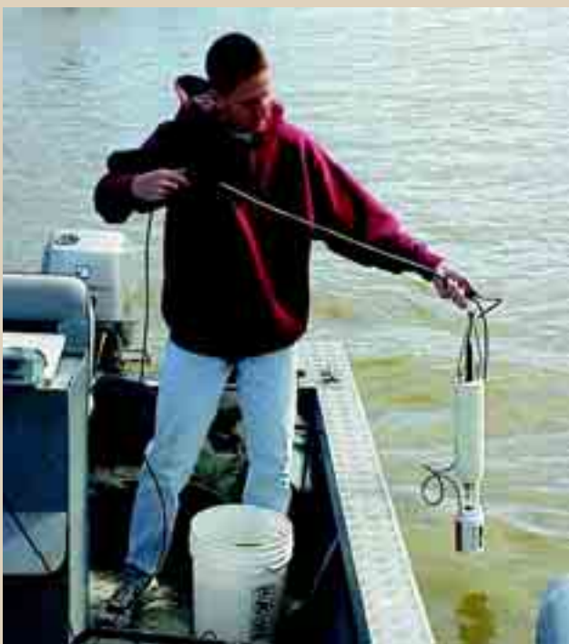
Figure 1. Recording conditions with a field water quality monitor.
