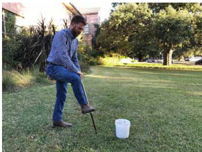
Take multiple soil samples across your lawn or planting bed to ensure a representation of the entire area.
